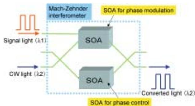
Fig. 4. Optical switch type: Cross phase modulation (XPM).
