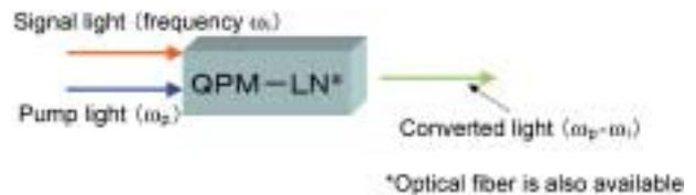
Fig. 7. Optical mixing type: Difference frequency generation (DFG).
