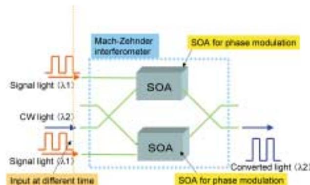
Fig. 5. Optical switch type: Differential phase modulation (DPM).
