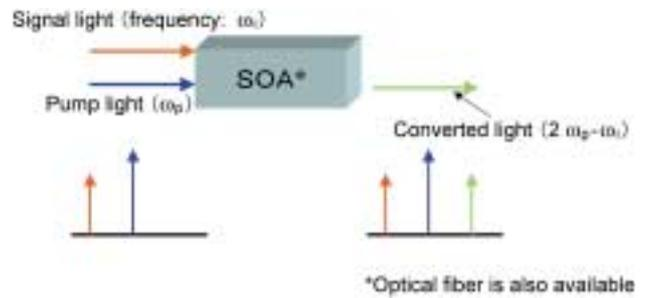
Fig. 6. Optical mixing type: Four wave mixing (FWM).
