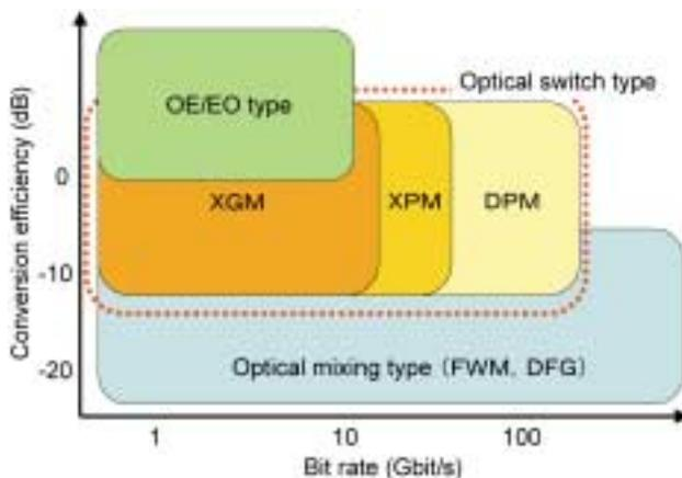
Fig. 2. Characteristics of wavelength conversion technologies.
