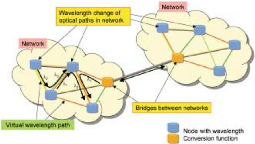
Fig. 1. Wavelength conversion technologies in photonic networks.
