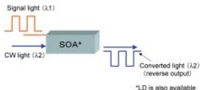
Fig. 3. Optical switch type: Cross gain modulation (XGM).
