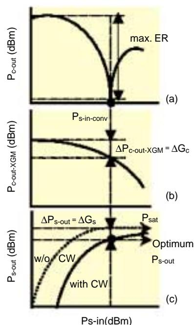
Fig. 8. Output power of (a) converted output signal  $P_{C-out}$  (XPM), (b) converted output signal  $P_{C-out-XGM}$  (XGM,  $I_{pc} = 0$  mA), (c) amplified signal  $P_{S-out}$ .
