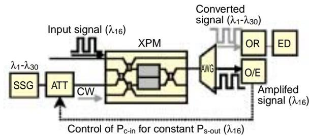
Fig. 9. Experimental setup for variable XPM wavelength conversion.
