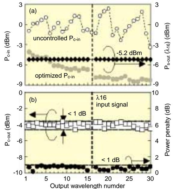
Fig. 10. Results of variable wavelength conversion. (a) Left axis: uncontrolled and optimized input CW power and Right axis: monitor signal power. (b) Left axis: converted output signal power Right axis: back-to-back power penalty.
