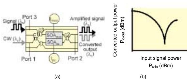
Fig. 1. (a) Schematic of XPM-WC, (b) wavelength conversion curve.
