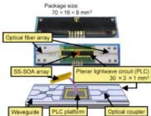
Fig. 4. Hybrid XPM module and device assembly.
