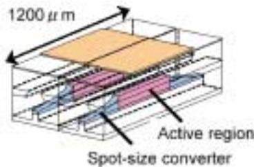
Fig. 3. Structure of SS-SOA array.
