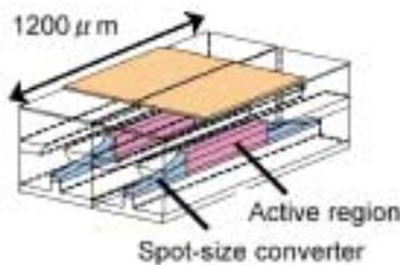
Fig. 3. Structure of SS-SOA array.
