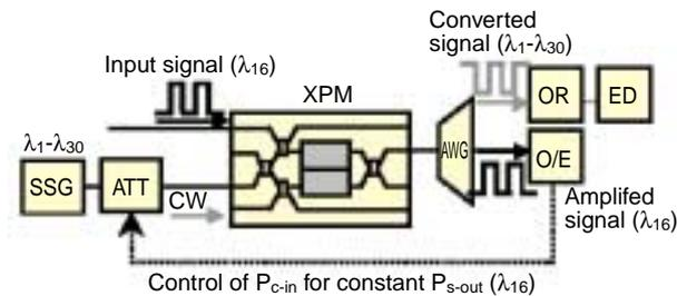
Fig. 9. Experimental setup for variable XPM wavelength conversion.
