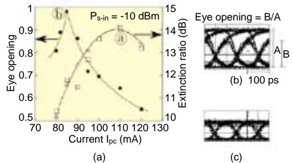
Fig. 5. (a) Dependence of eye opening and extinction ratio on current  $I_{\text{pc}}$ , (b) eye Pattern at operation point, (c) eye Pattern at operation point.
