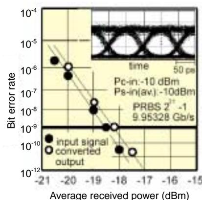
Fig. 6. 10-Gbit/s bit error characteristics and output eye pattern.
