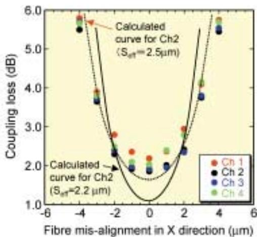
Fig.3. Measured and calculated coupling losses of MOCA.
