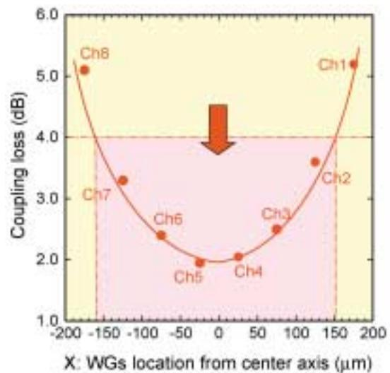
Fig. 5. Coupling losses of MOCA for an 8-ch waveguide array.
