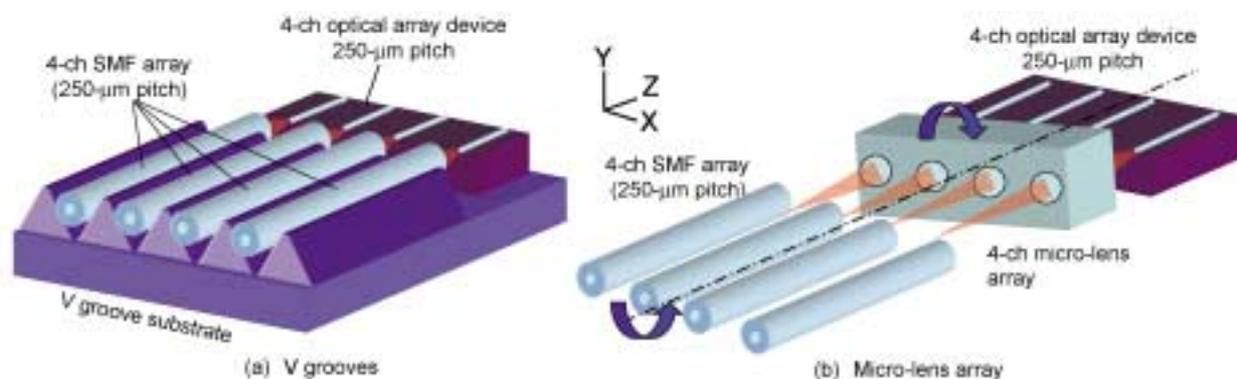
Fig. 1. Conventional multichannel optical coupling techniques.
