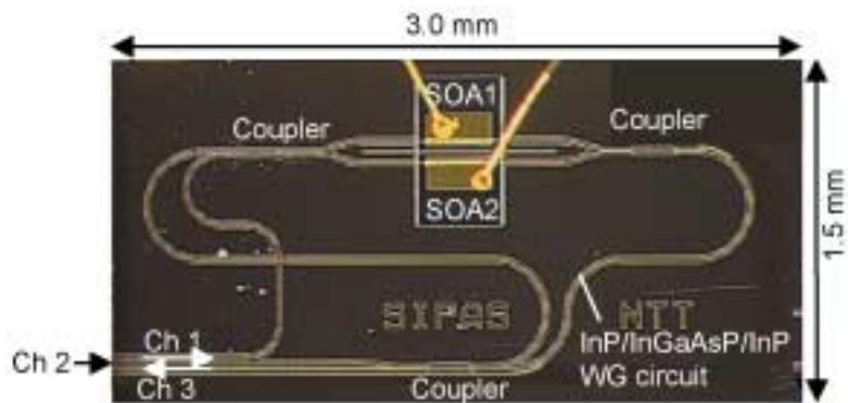
Fig. 6. Photograph of a SIPAS chip.
