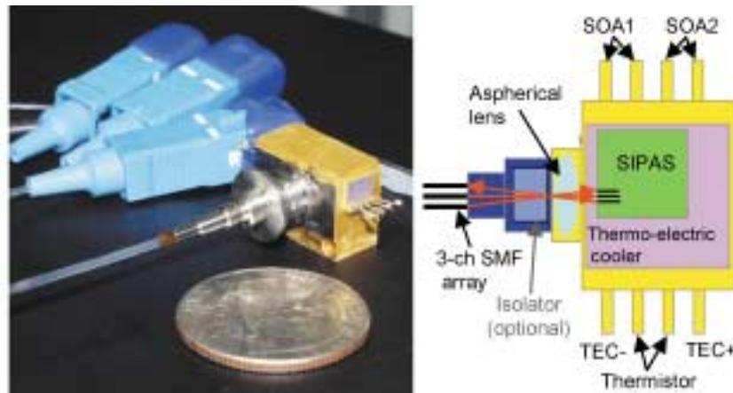
Fig. 7. Photograph and schema of the SIPAS module with MOCA.
