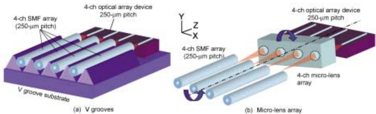
Fig. 1. Conventional multichannel optical coupling techniques.
