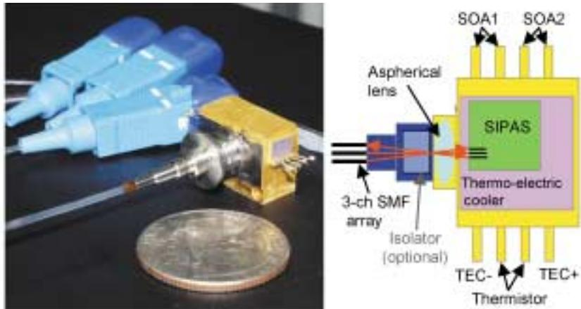
Fig. 7. Photograph and schema of the SIPAS module with MOCA.
