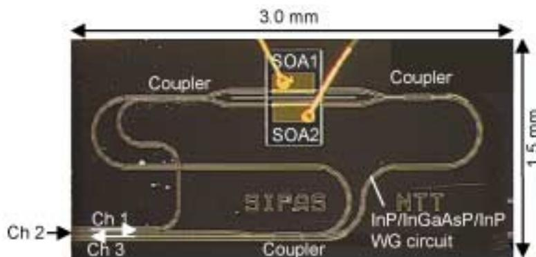
Fig. 6. Photograph of a SIPAS chip.
