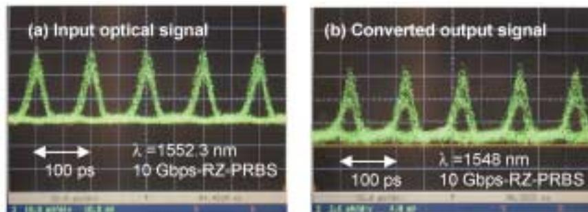
Fig. 8. Eye diagrams. (a) Input signal (1552.3 nm), (b) Conversion output (1548.0 nm).
