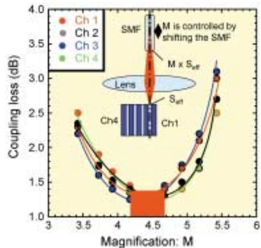
Fig. 4. Relation between coupling loss and magnification  $M$ .
