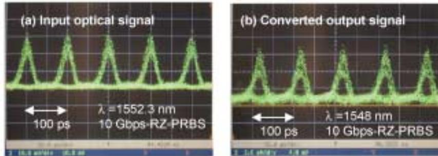
Fig. 8. Eye diagrams. (a) Input signal (1552.3 nm),
