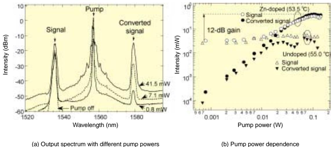
Fig. 6. Parametric amplification with pulsed pump.
