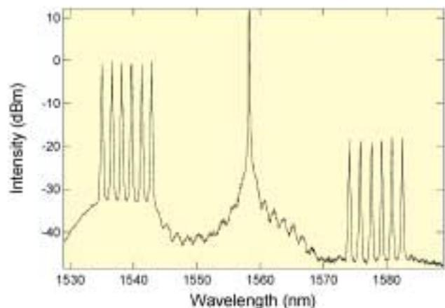
Fig. 2. Spectrum for multiple wavelength conversion with a cascade pump.
