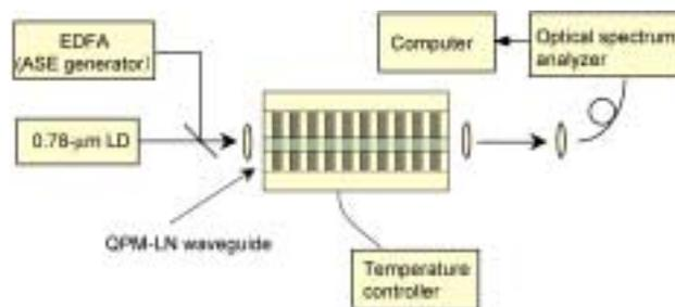
Fig. 4. Experimental setup for measuring optical damage.
