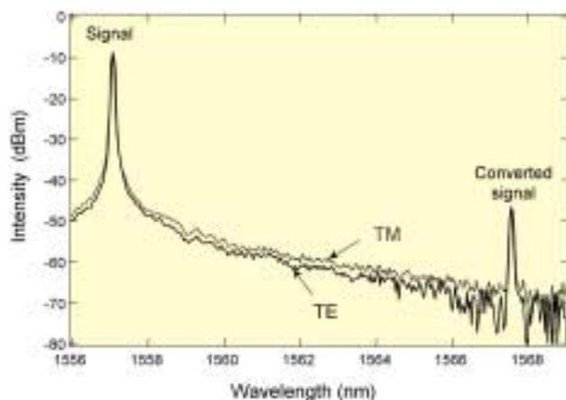
Fig. 9. DFG spectrum in a polarization-independent device.
