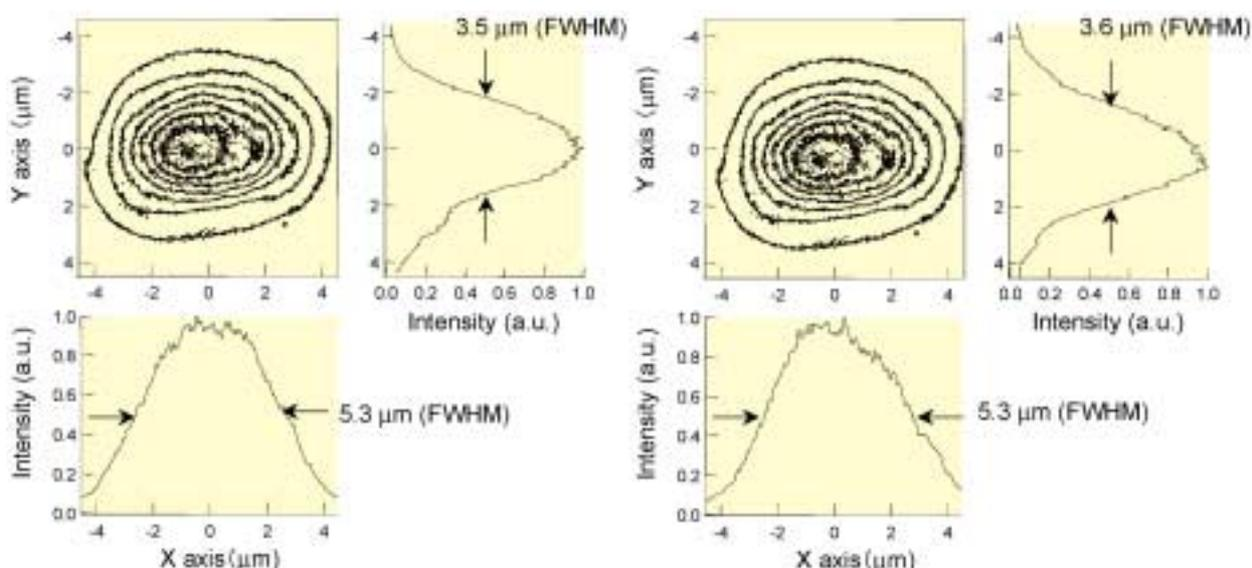
Fig. 7. Waveguide mode using an LPE-LN substrate (FWHM: full wave at half maximum).
