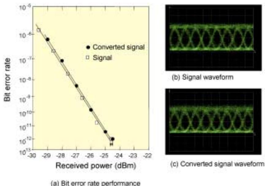
Fig. 3. Wavelength conversion characteristics for a 40-Gbit/s optical signal.
