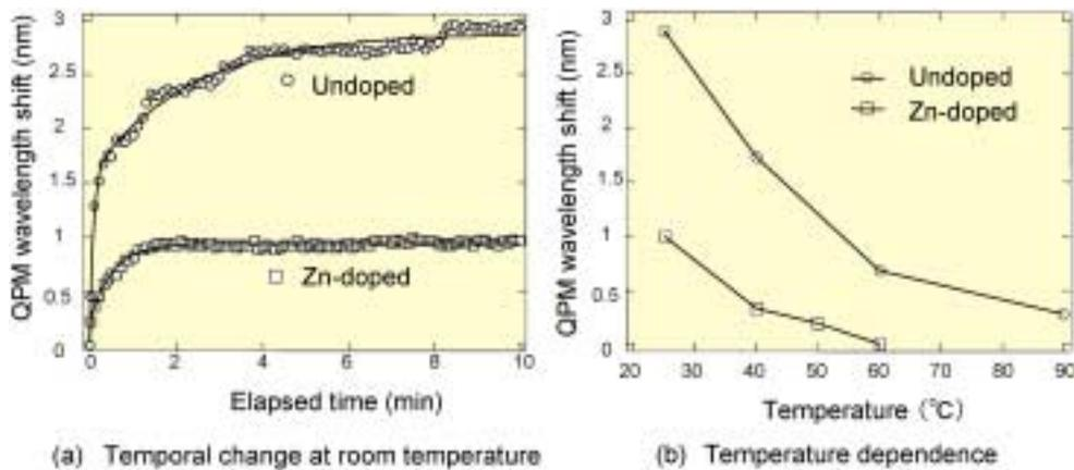
Fig. 5. Change in QPM wavelength caused by optical damage.
