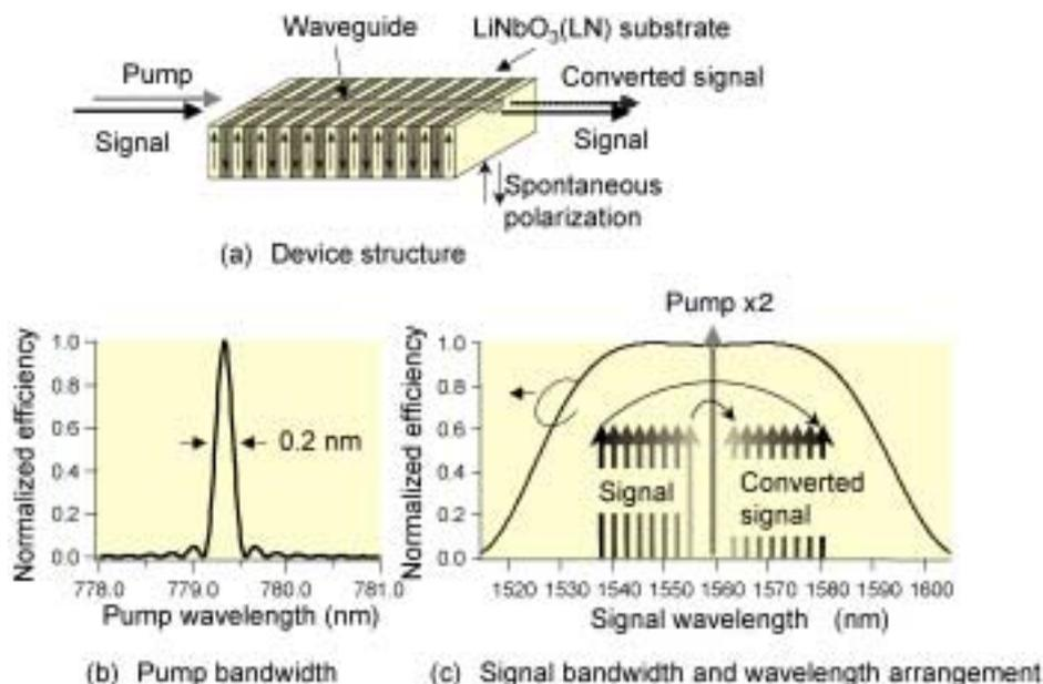
Fig.1. Structure and operating principle of a QPM-LN wavelength conversion device.
