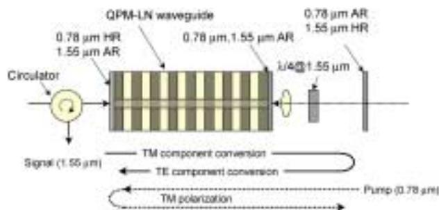
Fig. 8. Structure of a polarization-independent device with an LPE-LN waveguide. HR: highly reflective facet; AR: anti-reflection coated.
