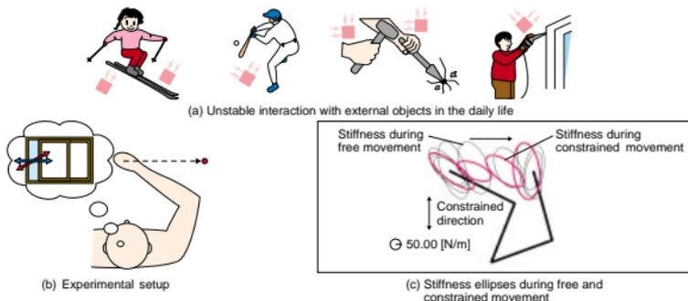
Fig. 3. Stiffness change during constrained movement.
