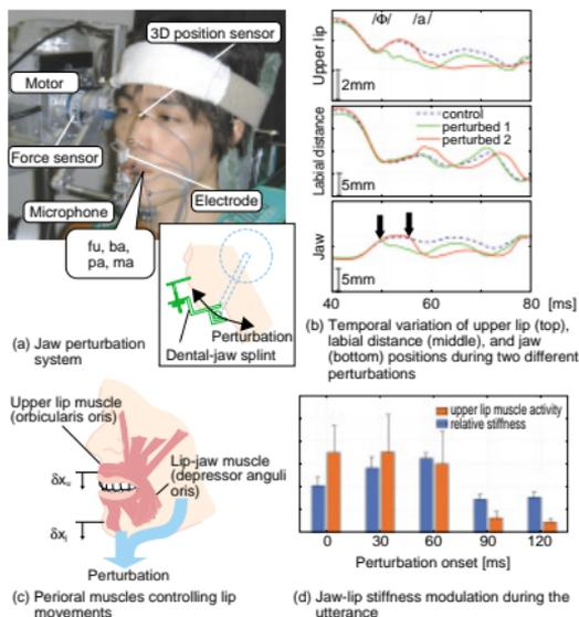
Fig. 4. Jaw-lip coordination for labial consonant production.
