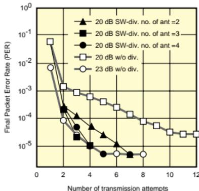
Fig. 2. Effect of cyclic-antenna-switching diversity (SW-div).
