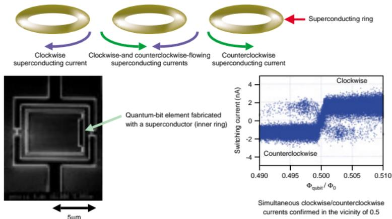
Fig. 2. Quantum-bit elements.
