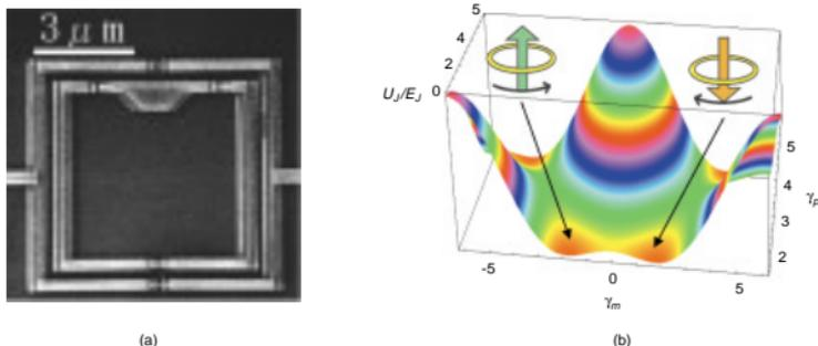
Fig. 1. (a) A scanning electron microscope photograph of a superconducting ring and a DC-SQUID as a readout device. (b) 3D plot of the potential energy of the qubit.
