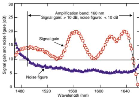
Fig. 5. Amplification characteristics of tellurite FRA.
