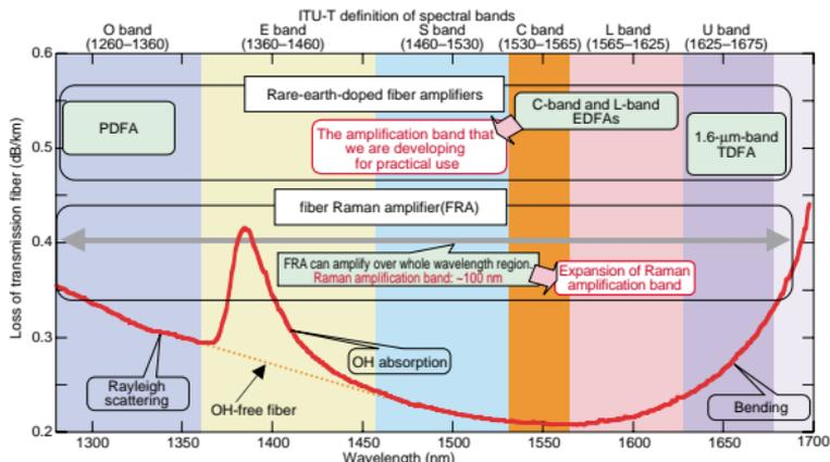
Fig. 1. Amplification bandwidth of each type of amplifier and loss spectrum of transmission fiber.
