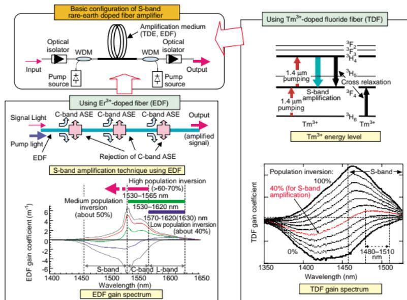
Fig. 2. S-band rare-earth doped fiber amplifiers.
