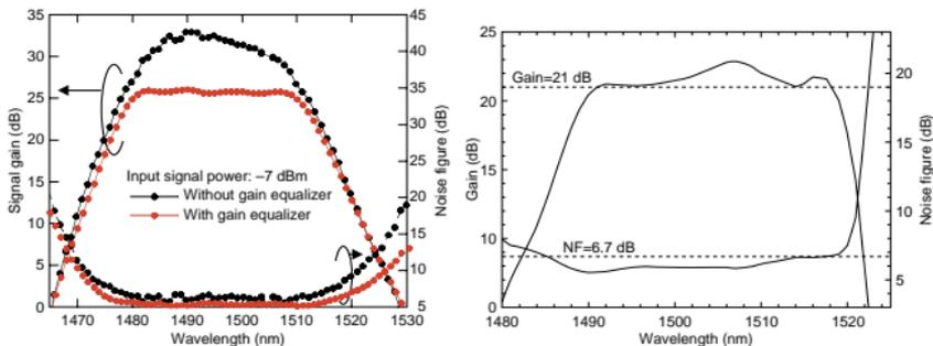
Fig. 3. (a) Amplification characteristics of TDFA, (b) Amplification characteristics of S-band EDFA.
