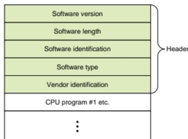
Fig. 10. Header information of the communication control program.
