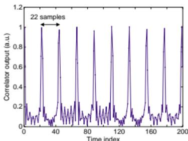
Fig. 12. Correlation output for wireless LAN mode.
