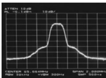
Fig. 13. Transmitter spectrum for PHS mode.
