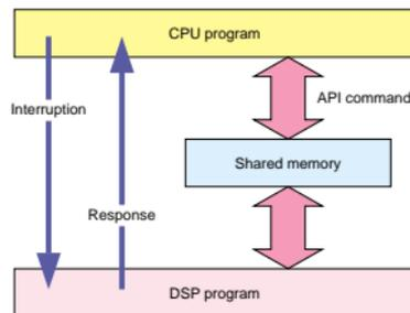
Fig. 7. API between CPU and DSP programs.
