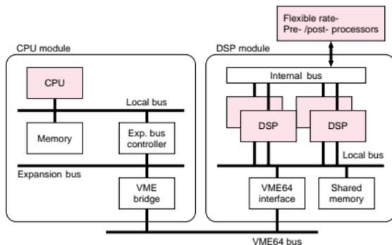
Fig. 2. Multiprocessor architecture.
