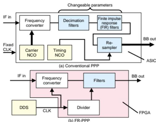
Fig. 3. Configurations of conventional PPP and FR-PPP (receiving blocks).
