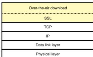
Fig. 8. Over-the-air download protocol stack.
