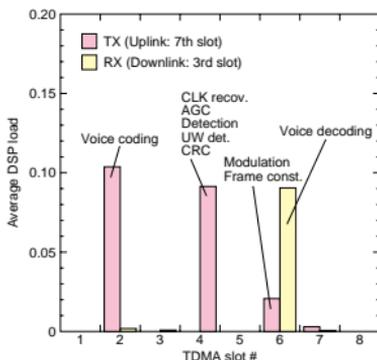
Fig. 19. Measured average DSP load of PS in each TDMA slot.
