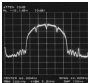
Fig. 11. Transmitter spectrum for wireless LAN mode.
