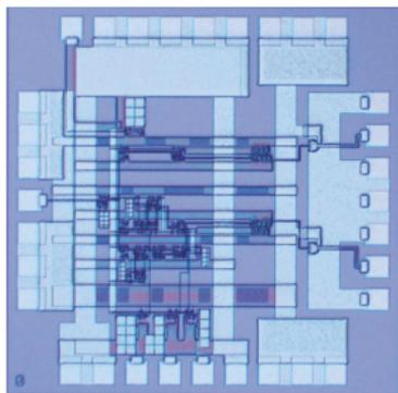
Fig. 15. Photograph of the variable frequency divider.
