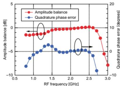
Fig. 6. Measured amplitude balance and quadrature phase error of the quadrature mixer for the demodulator.
