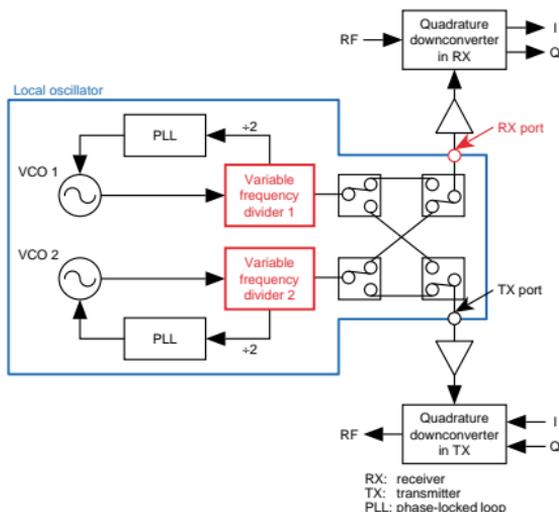
Fig. 13. Block diagram of the local oscillator architecture.
