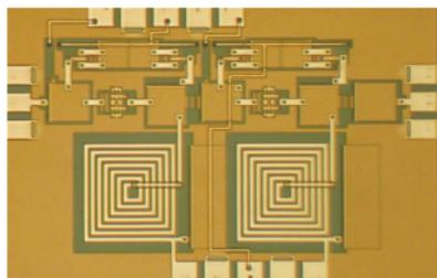
Fig. 9. Photograph of the low-noise variable-gain amplifier.
