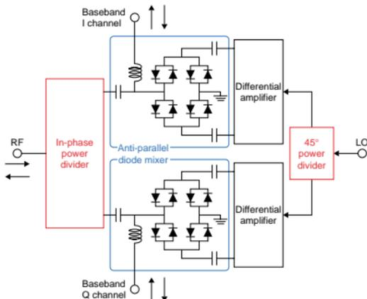
Fig. 2. Circuit configuration of the quadrature mixer.
