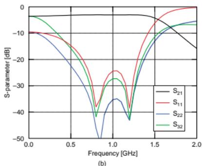
Fig. 4. In-phase power divider: (a) circuit configuration and (b) simulated S-parameters.
