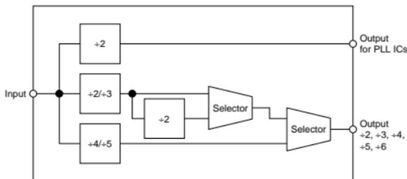
Fig. 14. Block diagram of the variable frequency divider.
