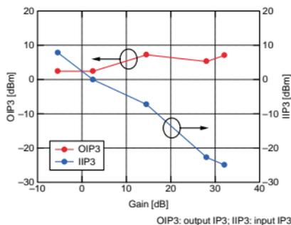
Fig. 12. Measured third intercept points of the low-noise variable-gain amplifier.
