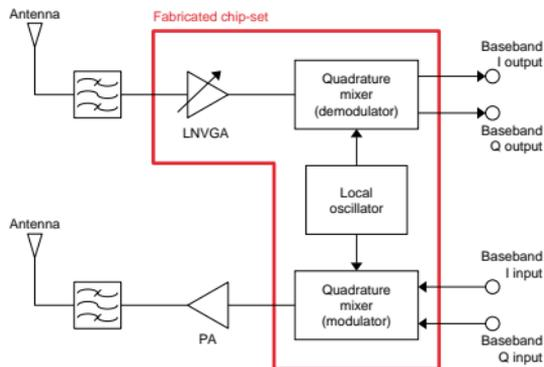
Fig. 1. Block diagram of the multi-band direct conversion transceiver.
