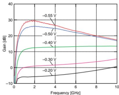
Fig. 10. Measured gain response of the low-noise variable-gain amplifier.
