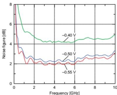
Fig. 11. Measured noise figure of the low-noise variable-gain amplifier.
