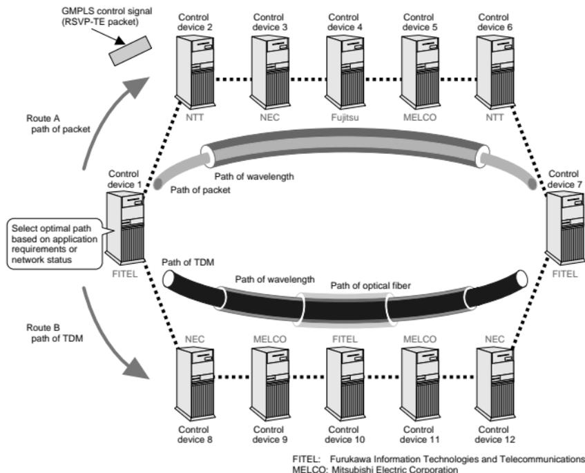
Fig. 1. Setup of GMPLS signaling experiment in multilayer network.
