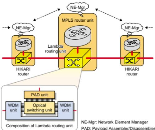
Fig. 2. Functional Components of HIKARI Router.
