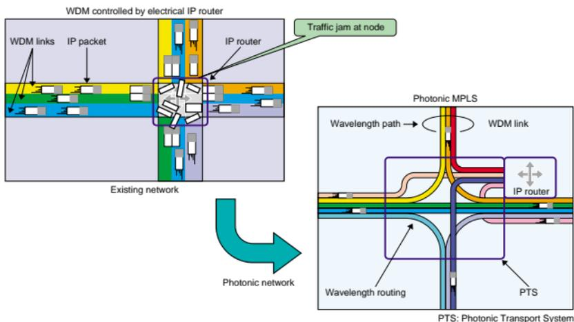
Fig. 1. Wavelength routing on photonic superhighway.
