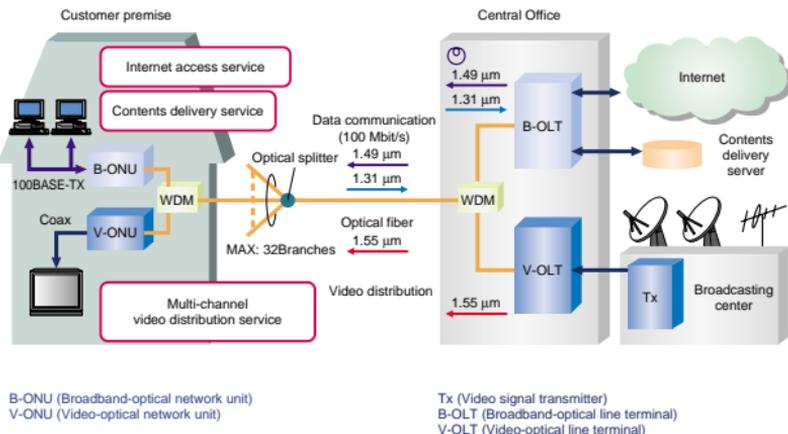
Fig. 1. Broadband passive optical network system (B-PON).
