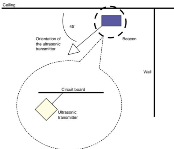
Fig. 4. Correct alignment of Cricket ultrasonic transmitter.
