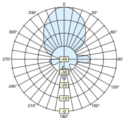
Fig. 3. Radiation pattern of an ultrasonic transmitter.
