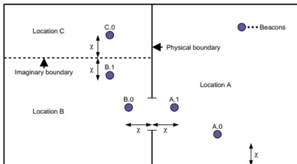
Fig. 2. Correct positioning of beacons.
