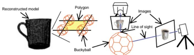
Fig. 1. 3-D data generation algorithm.
