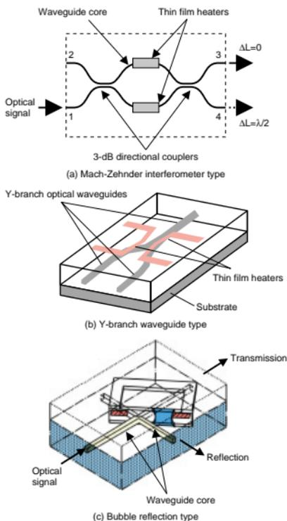
Fig. 3. Unit structure of optical waveguide type switch devices developed in NTT.
