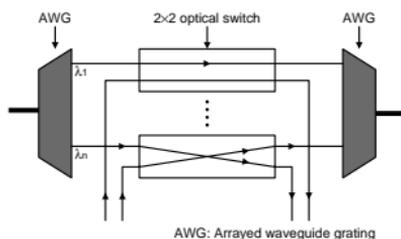
Fig. 2. Basic structure of OADM system.
