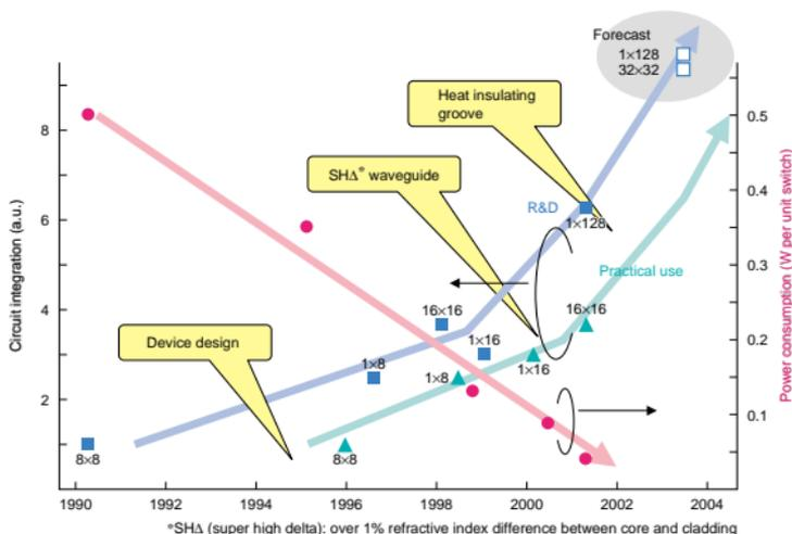
Fig. 4. Progress in optical circuit integration and power consumption in PLC switch devices.
