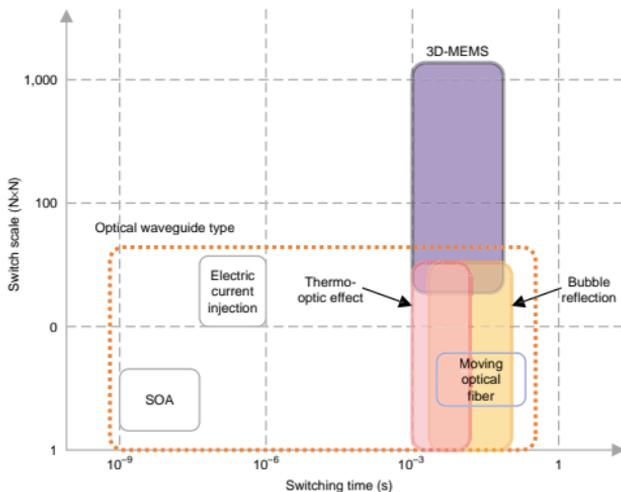
Fig. 5. Switch scale and switching time of various optical switch devices.
