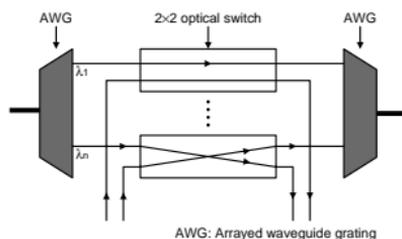
Fig. 2. Basic structure of OADM system.
