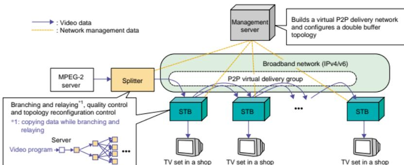
Fig. 5. System configuration.
