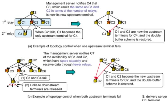
Fig. 4. Example of topology control after a terminal failure.
