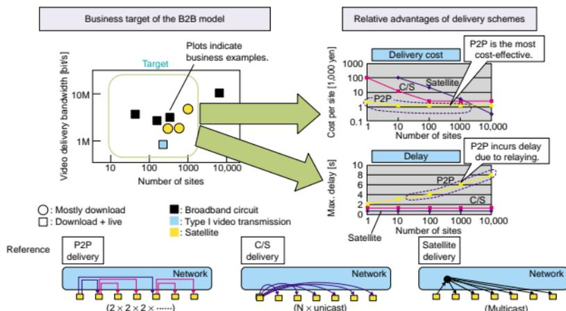
Fig. 2. Examples of B2B video delivery and the relative advantages of various delivery schemes.
