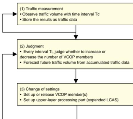
Fig. 5. Variable-capacity VCOP control procedure (VCOP: virtually concatenated optical path).
