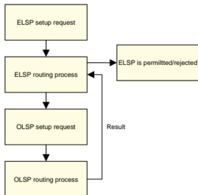
Fig. 7. Flow diagram of multi-layer routing.
