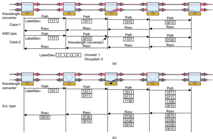
Fig. 4. Approaches based on signaling: (a) AND and (b) ALL types [10].
