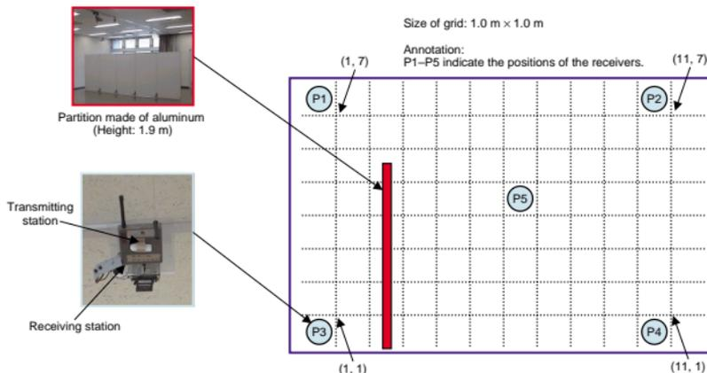
Fig. 7(a). Layout of experimental laboratory.
