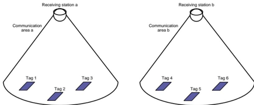
Fig. 2. Conventional active RFID tag system.
