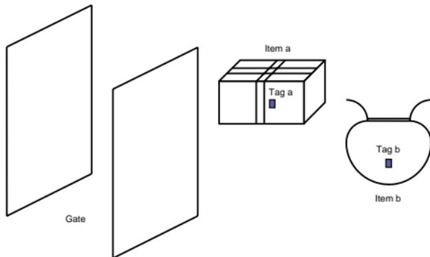
Fig. 1. Passive RFID tag system using gates.
