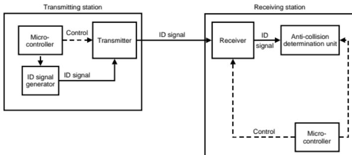
Fig. 5. Structures of the transmitting and receiving stations used in the locating system.
