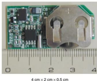
Fig. 6. Photograph of long-life active RFID tag.
