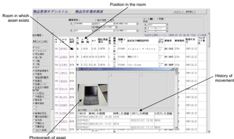
Fig. 8. Example of tracking of assets.
