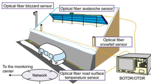
Fig. 4. Monitoring disasters involving snow and ice.
