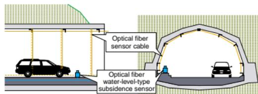
Fig. 6. Monitoring tunnels.
