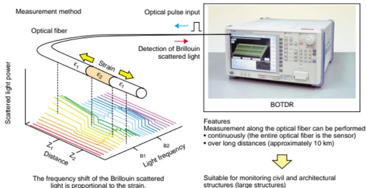
Fig. 1. Overview of system using the BOTDR method.
