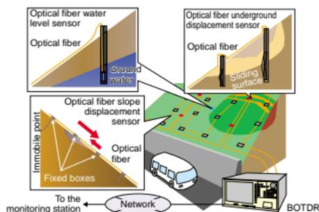
Fig. 3. Monitoring the collapse of a sloping surface layer.
