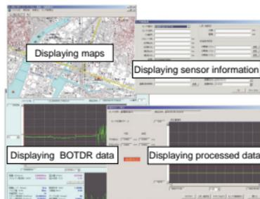
Fig. 7. Example screen-shot of road disaster monitoring system.
