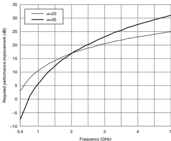
Fig. 4. Required performance improvement to achieve 100 Mbit/s from 2 Mbit/s at 2 GHz as a function of frequency.
