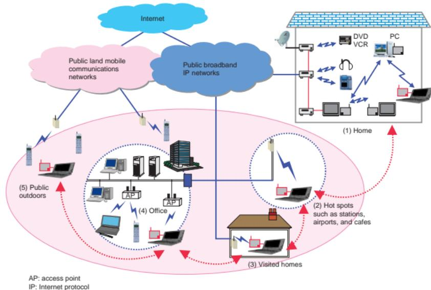
Fig. 1. Scenario for using future broadband mobile communications networks.
