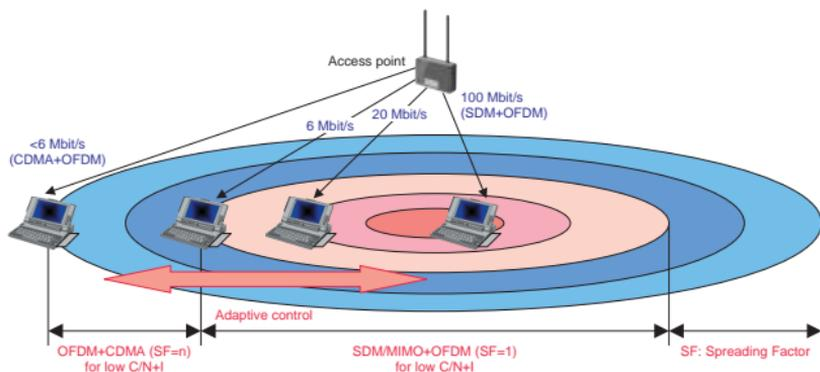
Fig. 6. Example of OFDM-based wireless access system using both SDM/MIMO and CDMA to maximize the frequency utilization efficiency.
