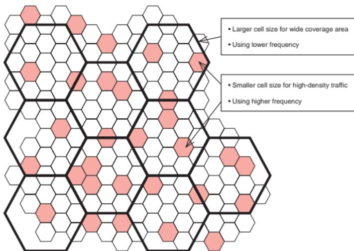
Fig. 5. Multi-layered cell concept for high-capacity and broadband mobile/nomadic systems.
