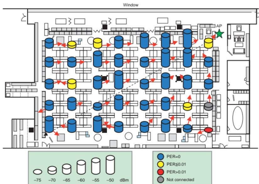
Fig. 4. Floor plan ( $38 \times 23$  m) and measured packet error rate (PER), received signal level, and signal arrival direction. (16QAM,  $R=3/4$ )
