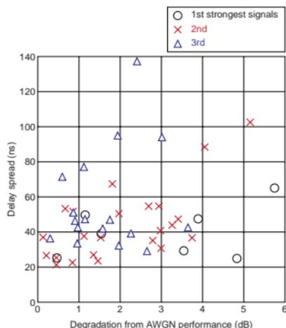
Fig. 6. Relationship between the degradation from the AWGN performance and measured delay spread.
