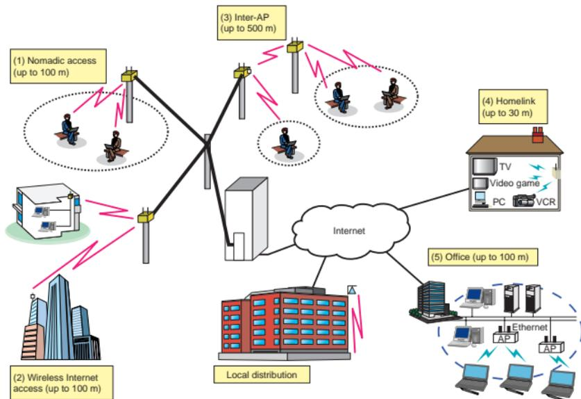
Fig. 1. Expected applications of wireless access systems using the quasi-millimeter wave band (AP: access point).
