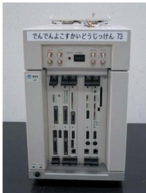
Fig. 3. Experimental equipment for measuring OFDM radio performance measurement in the 25-GHz band.
