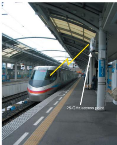
Fig. 2. Demonstration of a 25-GHz band WLAN system providing a broadband wireless connection between a train and a station.
