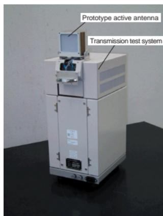
(b) Transmission test system using active integrated antenna
