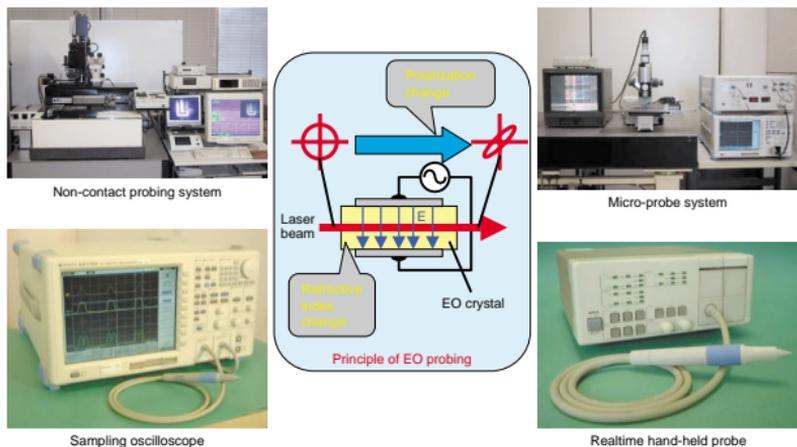
Fig. 1. Electro-optic (EO) probing systems.
