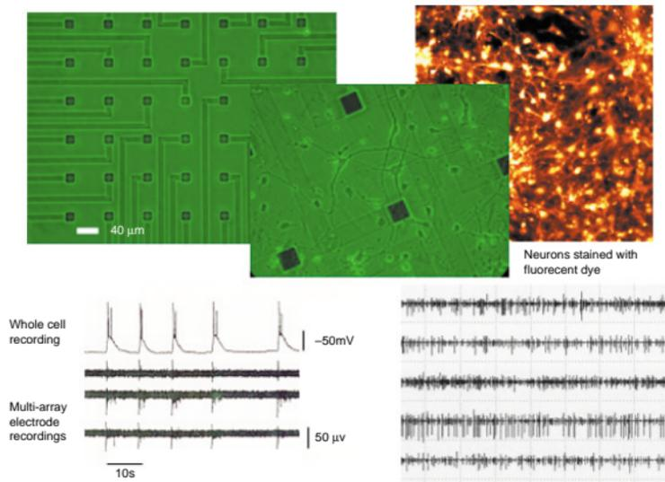
Fig. 7. Neural activity measurement using MEAS.
