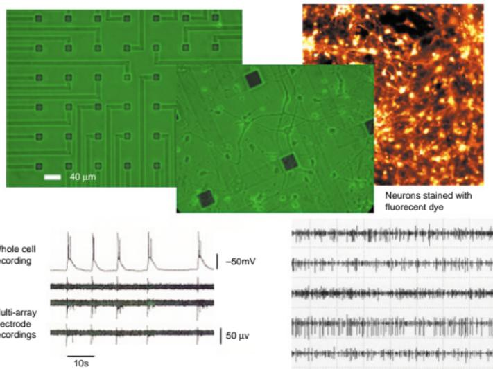
Fig. 7. Neural activity measurement using MEAS.
