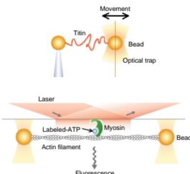
Fig. 1. Single molecular analysis using optical tweezers.
