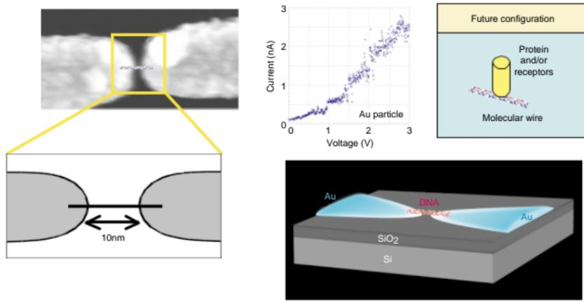
Fig. 9. Electrical conductivity measurement in single molecule using nano-gap electrode.
