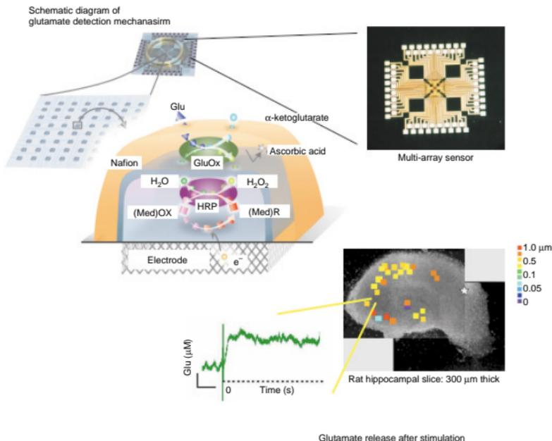
Fig. 8. Multi-site glutamate sensor based on MEAS.
