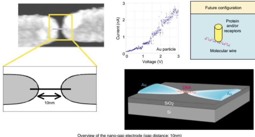
Fig. 9. Electrical conductivity measurement in single molecule using nano-gap electrode.
