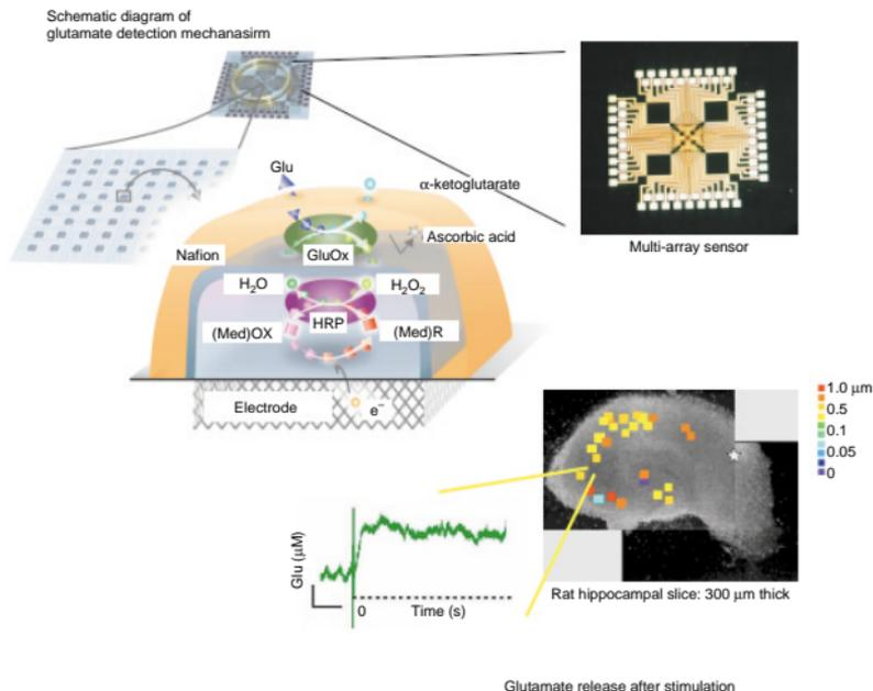
Fig. 8. Multi-site glutamate sensor based on MEAS.
