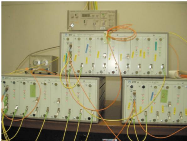
Fig. 2. Optical amplifiers for CWDM signals.
