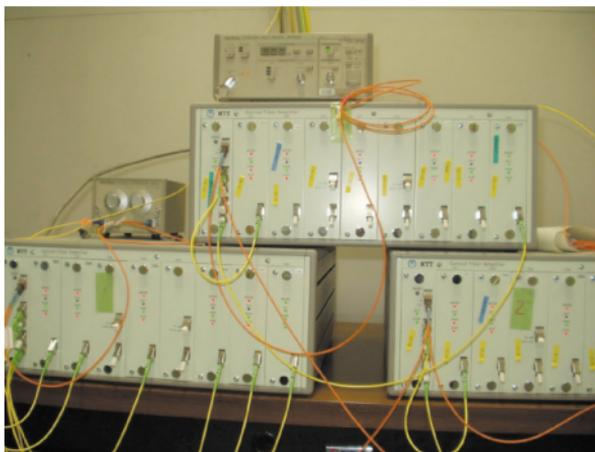
Fig. 2. Optical amplifiers for CWDM signals.
