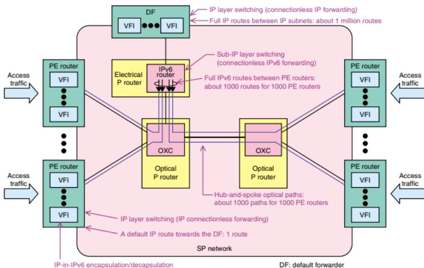
Fig. 7. IP-in-IPv6 overlay networking technology.
