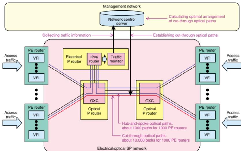
Fig. 8. Cut-through optical path control technology.
