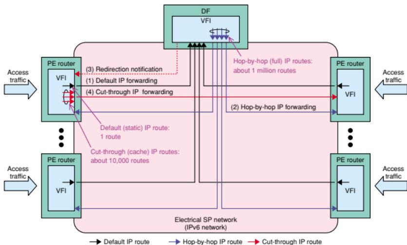
Fig. 9. Cut-through IP forwarding technology.
