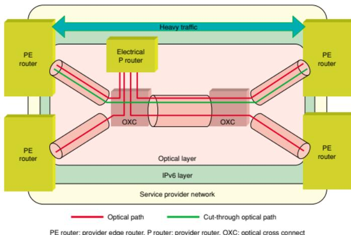
Fig. 1. Cut-through optical path.
