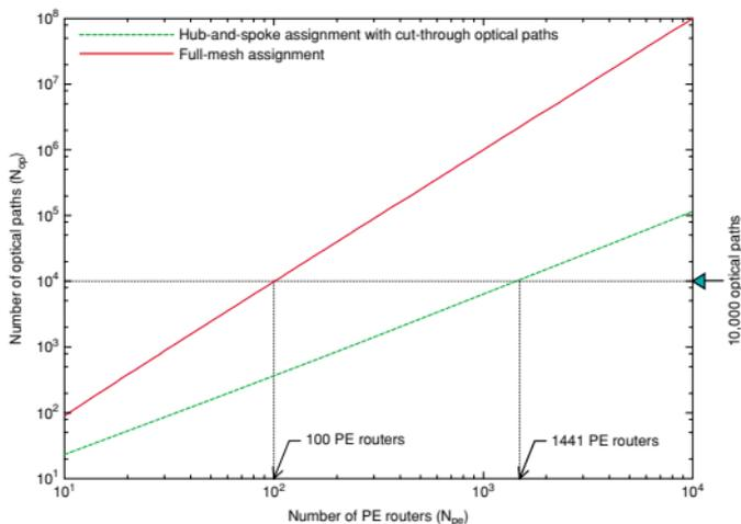
Fig. 6. Comparison of the number of optical paths.
