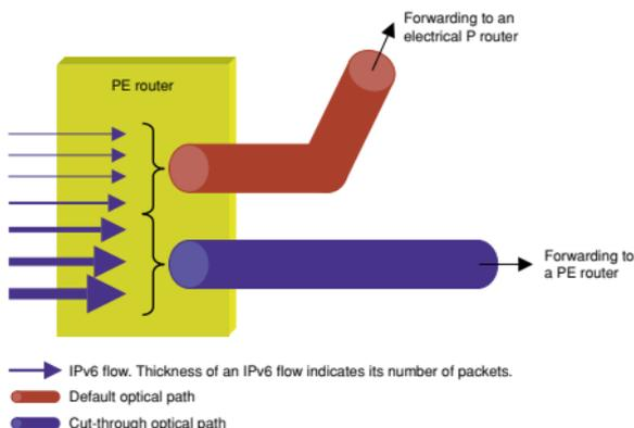
Fig. 3. Mapping IPv6 flows to optical paths.
