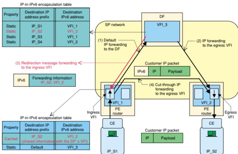
Fig. 3. Redirection control scheme.
