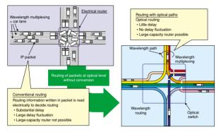
Fig. 7. Routing with optical paths.
