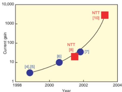
Fig. 3. Trend of current gain for nitride HBTs. Numbers in brackets are references.
