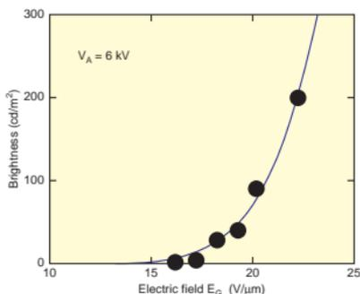
Fig. 8. Brightness as a function of the applied electric field strength  $E_G$ .
