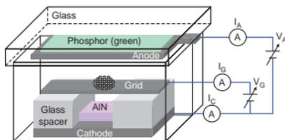
Fig. 6. Illustration of the AlN FED device developed by NTT Basic Research Laboratories.
