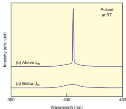
Fig. 11. Emission spectra of SELD obtained (a) below and (b) above the lasing threshold ( $J_{th}$ ) at room temperature (RT).
