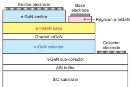
Fig. 1. Illustration of a typical HBT structure, which consists of an n-GaN emitter, a p-InGaN base, and an n-GaN collector.
