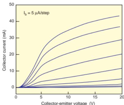
Fig. 2. Example of common emitter I-V characteristics of the HBT developed by NTT Basic Research Laboratories.
