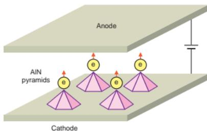
Fig. 5. Illustration of field emission from the tips of AlN pyramids.
