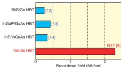
Fig. 4. Breakdown fields of HBTs composed of Si/SiGe [12], InGaP/GaAs [13], and InP/InGaAs [14] semiconductor material systems. Numbers in brackets are references.
