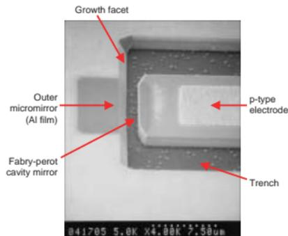
Fig. 10. Scanning electron micrograph showing a bird's-eye view of the fabricated SELD.
