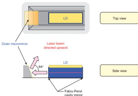
Fig. 9. Illustration of the new type SELD developed by NTT Basic Research Laboratories. The SELD consists of an HCLD with two Fabry-Perot cavity mirrors and an outer micromirror.
