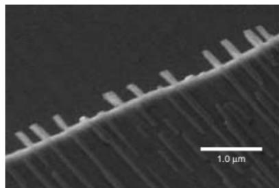
Fig. 8. SEM micrograph of fabricated InAs nanoscale cantilevers.
