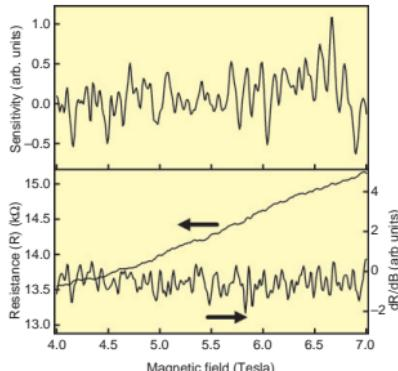
**Fig. 6.** (a) Measured sensitivity as a function of magnetic field. (b) Two-terminal resistance ( $R$ ) and its derivative ( $dR/dB$ ) measured for the same device as functions of magnetic field.
