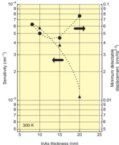
Fig. 3. Sensitivity and minimum detectable displacement of fabricated devices.
