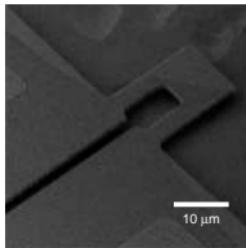
Fig. 2. Fabricated InAs/Al<sub>0.5</sub>Ga<sub>0.5</sub>Sb piezoresistive cantilever.
