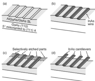
Fig. 7. Fabrication processes for InAs nanocantilevers using self-assembled growth.
