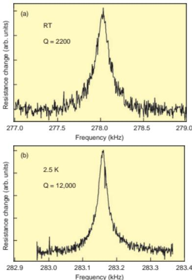
**Fig. 5.** Frequency responses obtained at (a) room temperature and (b) 2.5 K.
