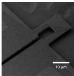
Fig. 2. Fabricated InAs/Al<sub>0.5</sub>Ga<sub>0.5</sub>Sb piezoresistive cantilever.
