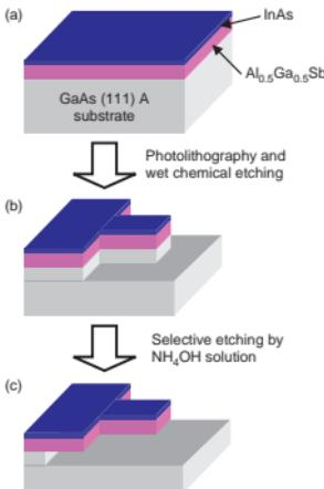
Fig. 1. InAs/AlGaSb piezoresistive cantilever fabrication processes.
