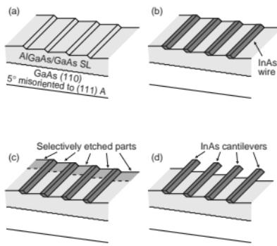
**Fig. 7.** Fabrication processes for InAs nanocantilevers using self-assembled growth.
