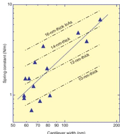
Fig. 9. Spring constants 100 nm from the clamped position evaluated for 14 different cantilevers. The dash-double-dotted line shows spring constants calculated from the cantilever dimensions and elastic constant of bulk InAs. The blue dotted line shows the least squares line fitting of obtained data.
