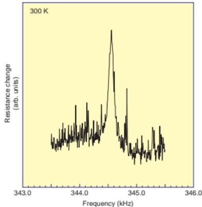
**Fig. 4.** Cantilever thermal vibration at 300 K detected by the resistance change in a fabricated InAs/Al<sub>0.5</sub>Ga<sub>0.5</sub>Sb piezoresistive cantilever.
