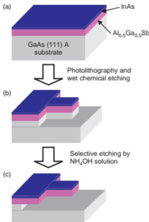
Fig. 1. InAs/AlGaSb piezoresistive cantilever fabrication processes.
