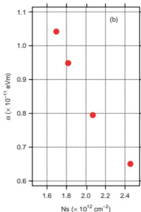
Fig. 2(b). Spin-orbit interaction parameter  $\alpha$  is plotted as a function of carrier concentration  $N_s$ , which is related to gate voltage  $V_g$ . Spin-orbit interaction can be controlled by the gate voltage.
