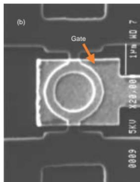
Fig. 3(b). SEM image of a fabricated spin-interference device.
