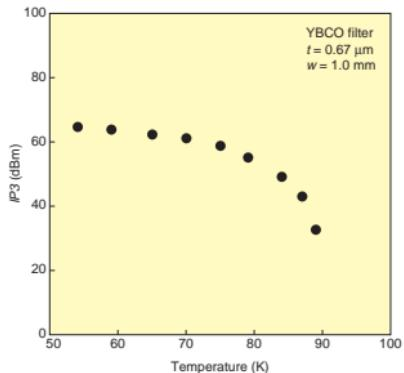
Fig. 5. Temperature dependence of the third-order intercept  $IP_3$  for a 3-pole microstrip bandpass filter fabricated on a film of  $\text{YBa}_2\text{Cu}_3\text{O}_7$  (YBCO) with thickness  $t = 0.67 \mu\text{m}$  and line width  $w = 1.0 \text{ mm}$ .
