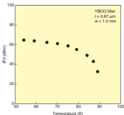
Fig. 5. Temperature dependence of the third-order intercept  $IP_3$  for a 3-pole microstrip bandpass filter fabricated on a film of  $\text{YBa}_2\text{Cu}_3\text{O}_7$  (YBCO) with thickness  $t = 0.67 \mu\text{m}$  and line width  $w = 1.0 \text{ mm}$ .
