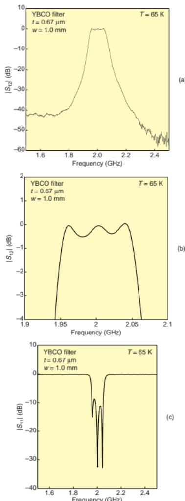
Fig. 3. Frequency dependences of (a)  $|S_{12}|$ , (b)  $|S_{11}|$  in the passband region and (c)  $|S_{11}|$  measured at 65 K for a 3-pole microstrip bandpass filter fabricated on a film of  $\text{YBa}_2\text{Cu}_3\text{O}_7$  (YBCO) with thickness  $t = 0.67 \mu\text{m}$  and line width  $w = 1.0 \text{ mm}$ .
