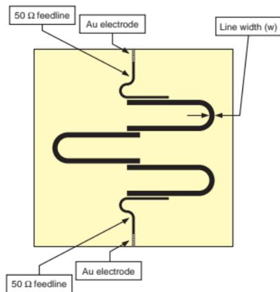
Fig. 2. Layout of a 3-pole microstrip bandpass filter composed of resonators with line width  $w$  and feed lines with the characteristic impedance of  $50 \Omega$ ; electrodes formed by Au evaporation.
