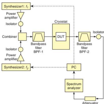
Fig. 1. Schematic diagram of experimental setup for third-order intermodulation measurements of a superconducting bandpass filter, labeled DUT (device under test).
