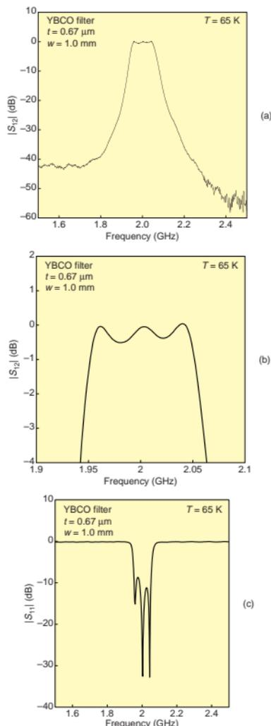
Fig. 3. Frequency dependences of (a)  $|S_{12}|$ , (b)  $|S_{12}|$  in the passband region and (c)  $|S_{11}|$  measured at 65 K for a 3-pole microstrip bandpass filter fabricated on a film of  $\text{YBa}_2\text{Cu}_3\text{O}_7$  (YBCO) with thickness  $t = 0.67$   $\mu\text{m}$  and line width  $w = 1.0$  mm.
