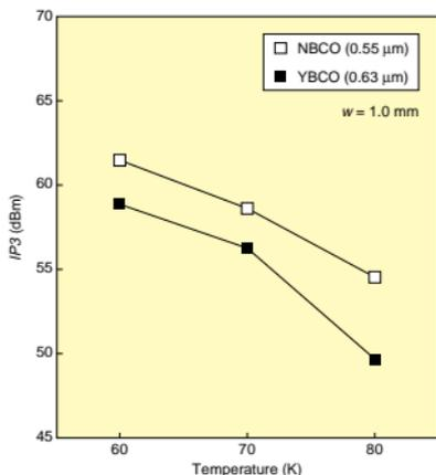
Fig. 7. Temperature dependences of the third-order intercept  $IP_3$  for 3-pole microstrip bandpass filters with line width  $w = 1.0$  mm fabricated on a film of  $\text{NdBa}_2\text{Cu}_3\text{O}_7$  (NBCO) grown by molecular-beam epitaxy with thickness  $t = 0.55$   $\mu\text{m}$  and a commercially obtained film of  $\text{YBa}_2\text{Cu}_3\text{O}_7$  (YBCO) with  $t = 0.63$   $\mu\text{m}$ .
