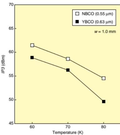
Fig. 7. Temperature dependences of the third-order intercept  $IP_3$  for 3-pole microstrip bandpass filters with line width  $w = 1.0$  mm fabricated on a film of  $\text{NbBa}_2\text{Cu}_3\text{O}_7$  (NBCO) grown by molecular-beam epitaxy with thickness  $t = 0.55$   $\mu\text{m}$  and a commercially obtained film of  $\text{YBa}_2\text{Cu}_3\text{O}_7$  (YBCO) with  $t = 0.63$   $\mu\text{m}$ .
