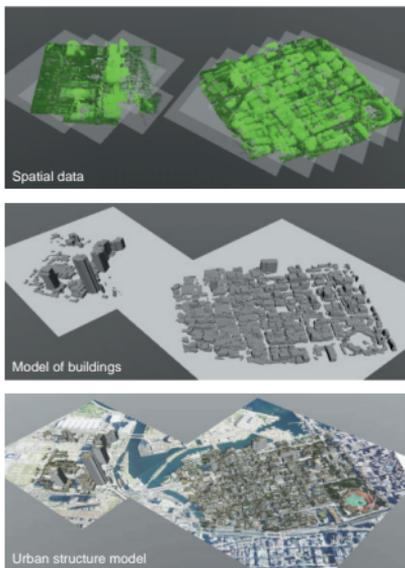
Fig. 6. Urban structural model produced from HD video.
