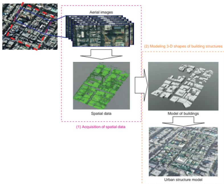
Fig. 1. Overview of 3-D model reconstruction from aerial images.
