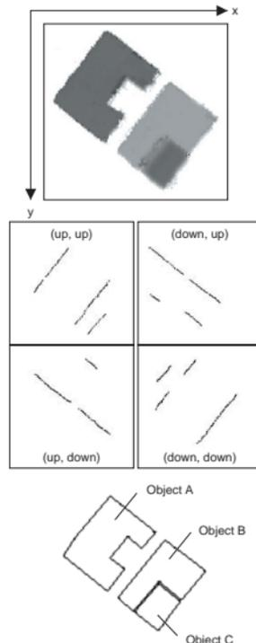
Fig. 9. Edge analysis and classification method.
