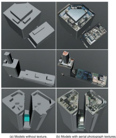
Fig. 12. Example of adding upper surface textures to building models.
