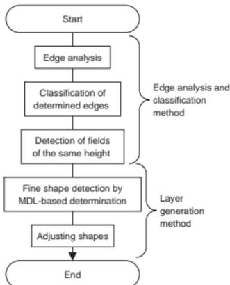
Fig. 8. Algorithm for detecting 2-D building shapes.
