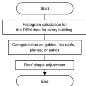
Fig. 10. Detection of a roof shape.
