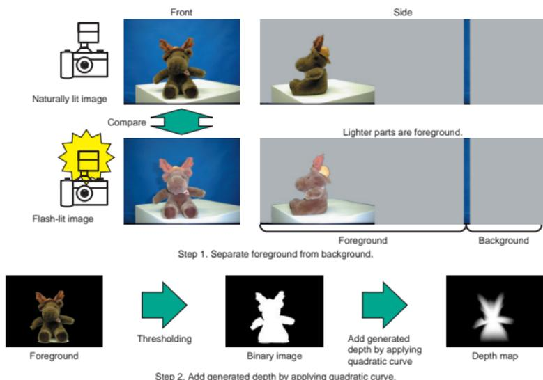
Fig. 2. Schematic diagram of REAL.
