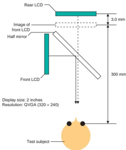
Fig. 8. Setup of subjective test using a depth-fused 3-D display.
