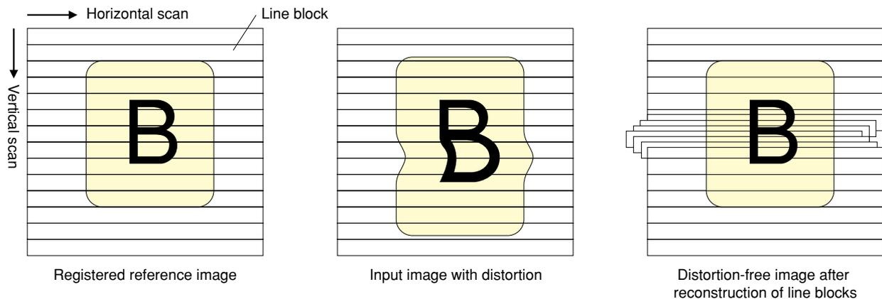
Fig. 3. Line-block distortion reduction method for pattern-matching inspection.
