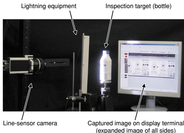
Fig. 2. Capturing images using a line-sensor camera.
