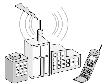
Fig. 3. Radio base stations need to be protected against lightning.
