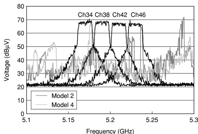
Fig. 5. Signal power of 5.2-GHz-band wireless LAN.
