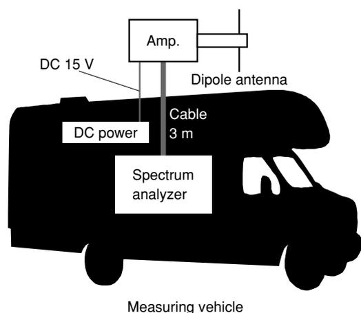
Fig. 1. Setup of measuring electromagnetic environment.
