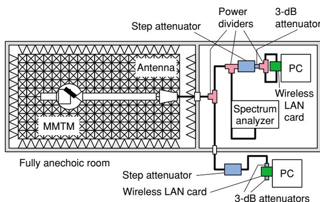
Fig. 6. Setup for measuring interference characteristics.
