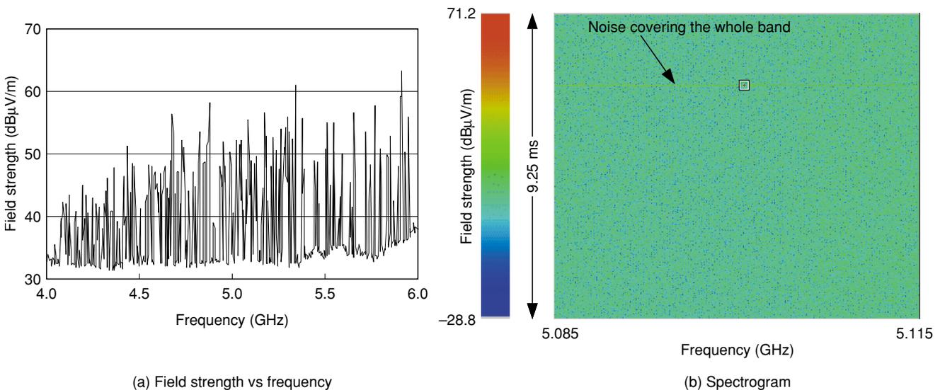
Fig. 4. Electromagnetic field strength measured at drugstore #2.
