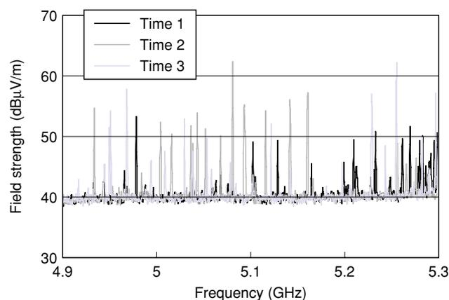
Fig. 3. Outdoor electric field intensity (changes over time).
