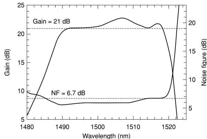
Fig. 5(b). Gain and noise figure spectra of S-band EDFA.
