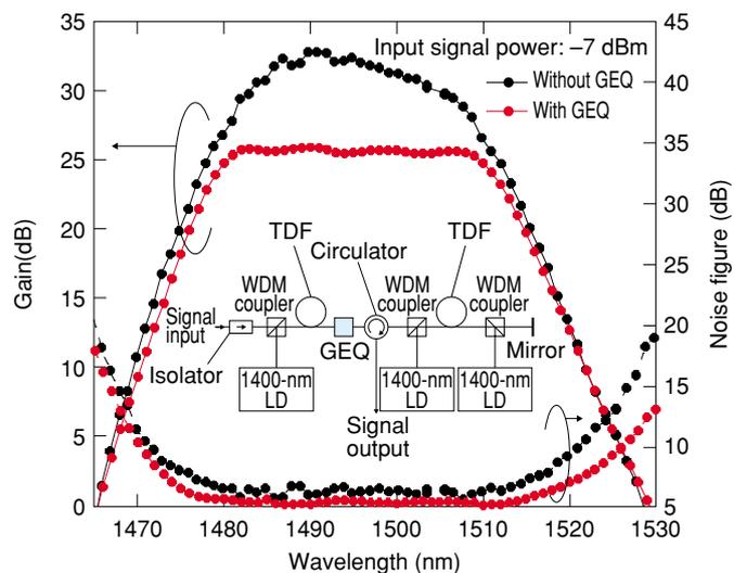
Fig. 3(c). Amplification characteristics of S-band TDFA.
