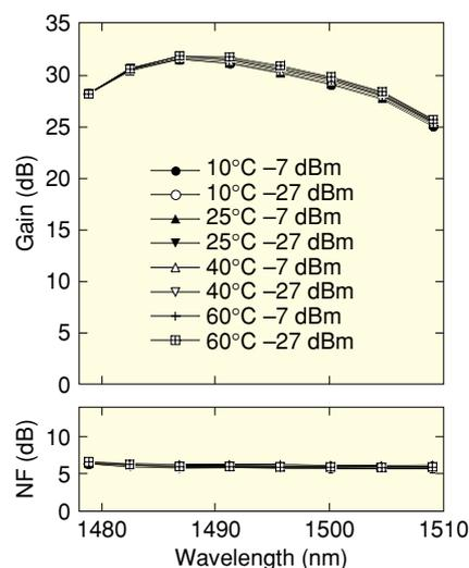
Fig. 4(c). Gain spectra and noise figures (NFs) when the gain control unit was operating against a total input signal power of  $-27$  to  $-7$  dBm and a temperature of 10 to  $60$  °C.
