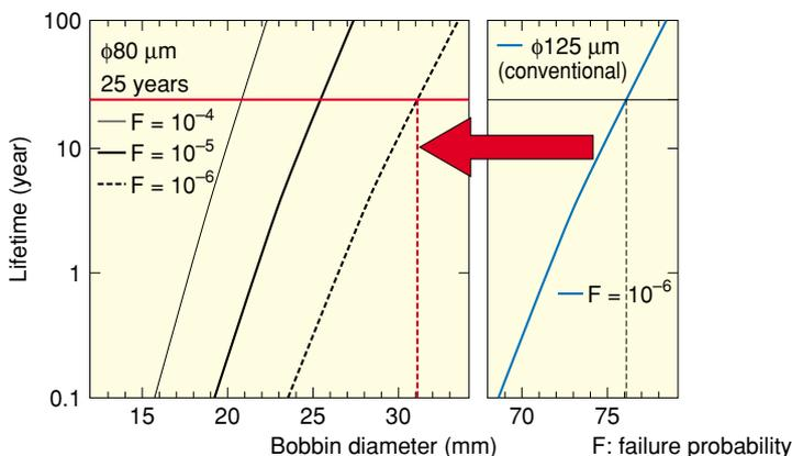
Fig. 2(b). Estimated lifetime versus bobbin diameter.
