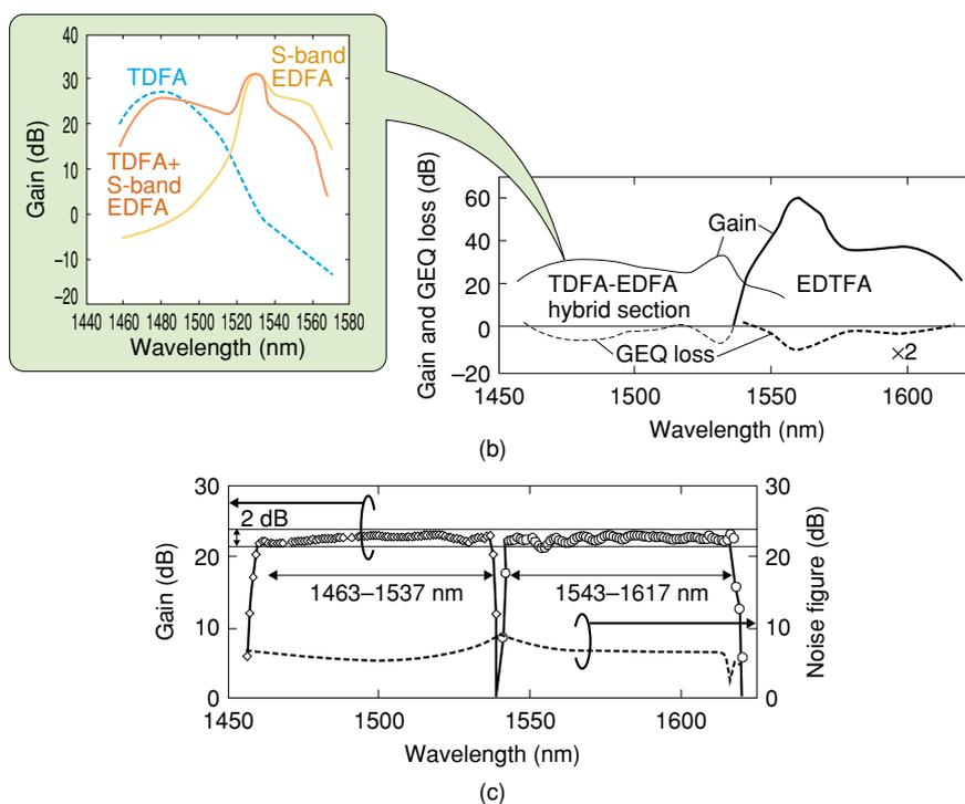
Fig. 6. Amplification characteristics (b) without GEQ and (c) with GEQ.
