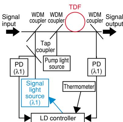
Fig. 4(b). Configuration of gain control unit for TDFA.
