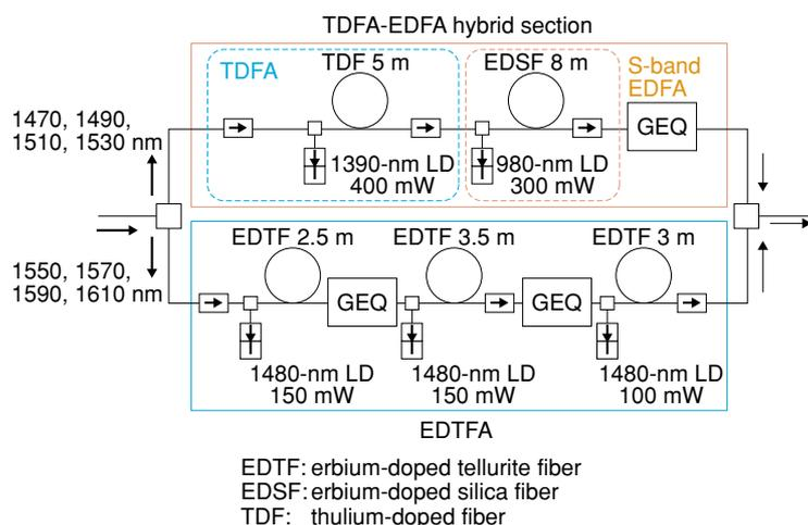
Fig. 6(a). Configuration of CWDM amplifier.
