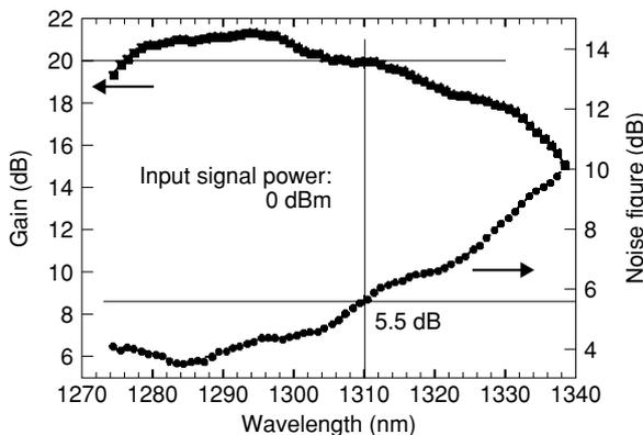
Fig. 1(c). Amplification characteristics of PDFA with our developed fluoride fiber.
