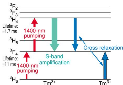
Fig. 3(a). Energy diagram of  $\text{Tm}^{3+}$ .
