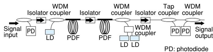
Fig. 1(b). Configuration of PDFA with our developed fluoride fiber.
