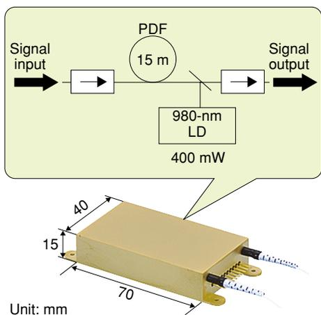
Fig. 2(a). Configuration and overview of gain block employed with our developed fluoride fiber.
