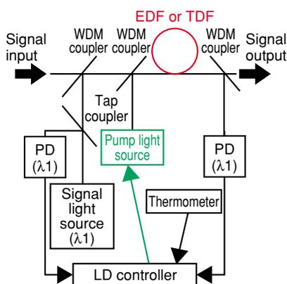
Fig. 4(a). Configuration of gain control unit for EDFA.
