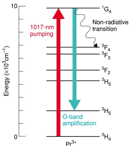
Fig. 1(a). Energy diagram of  $\text{Pr}^{3+}$ .
