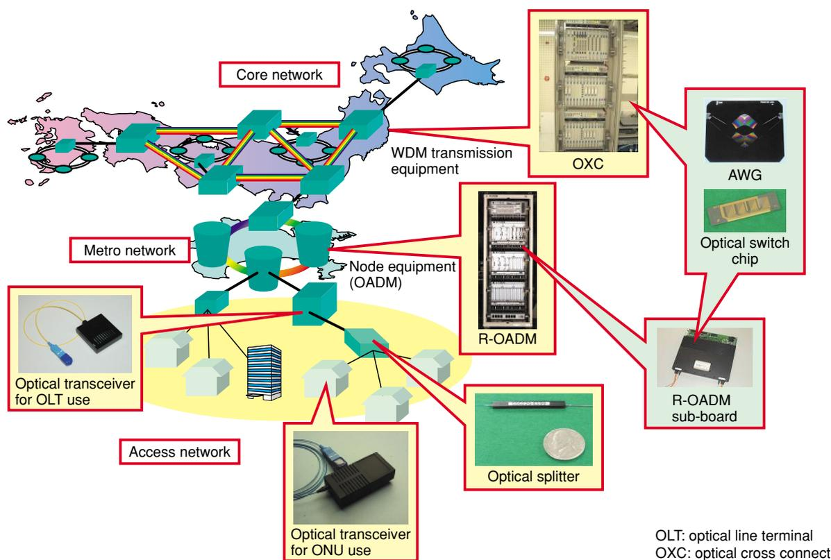
Fig. 1. Optical devices for network support.
