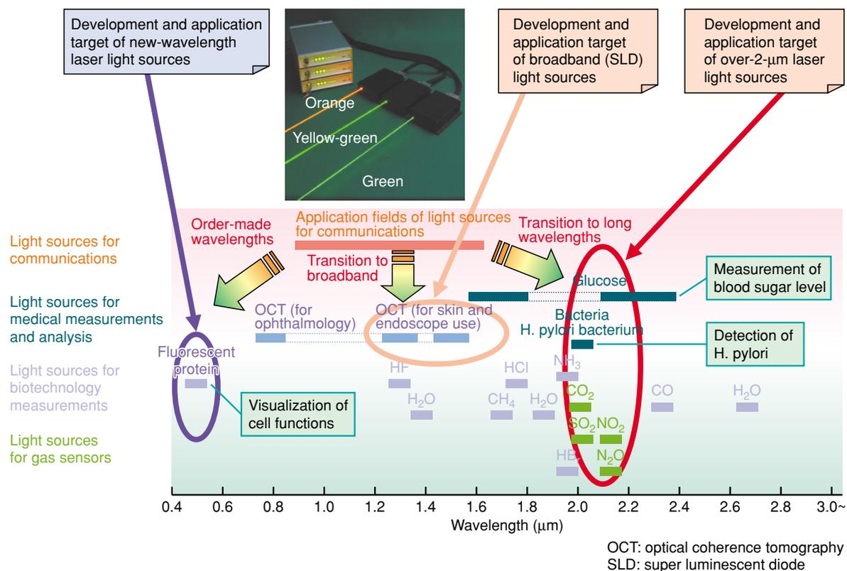
Fig. 3. Developing new application areas for optical devices: biotechnology/medical measurements and gas sensors.
