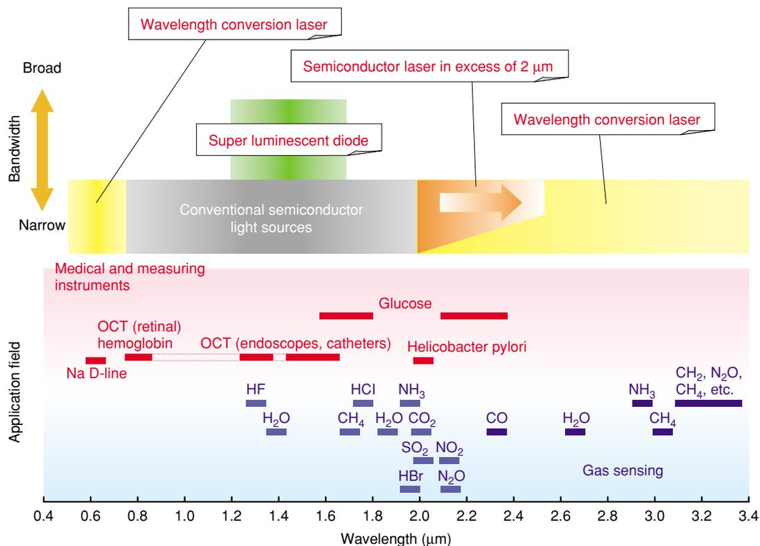
Fig. 1. Application fields and bandwidths of the new light sources.
