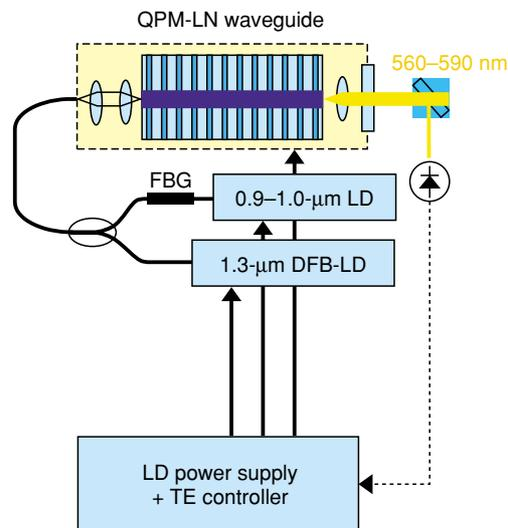
Fig. 6. Structure of the yellow laser.
