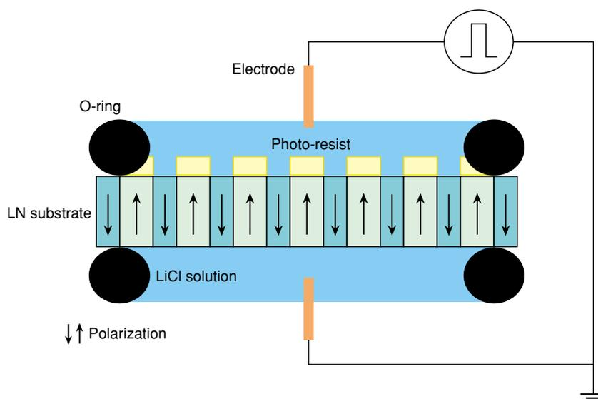
Fig. 3. Electrical poling method.
