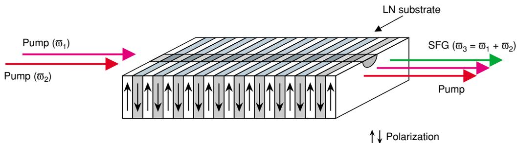
Fig. 2. Structure of QPM-LN device.
