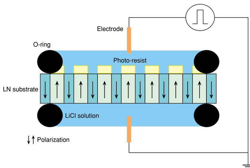
Fig. 3. Electrical poling method.
