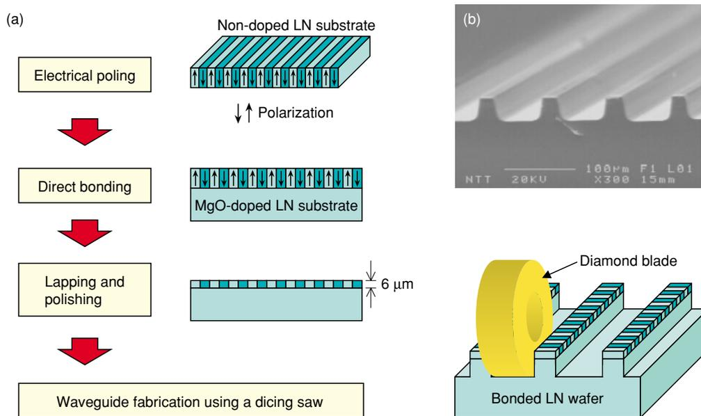
Fig. 5. Direct-bonded ridge waveguide fabrication process (a) and microscope photograph of ridge waveguide (b).
