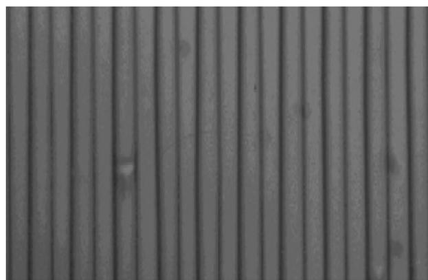
Fig. 4. Microscope photograph of periodically poled structure.
