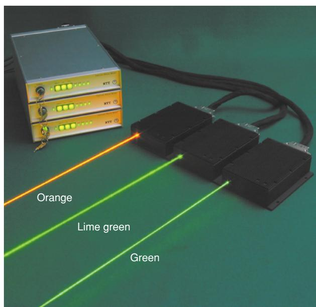
Fig. 7. Photograph of three yellow lasers with their power supplies (orange: 589 nm, lime green: 560 nm, green: 543 nm).
