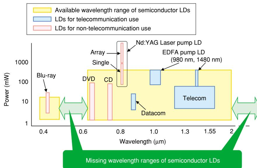
Fig. 1. Comparison of semiconductor LDs.
