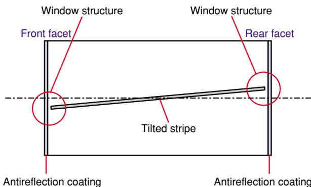
Fig. 1. Schematic structure of our SLD.
