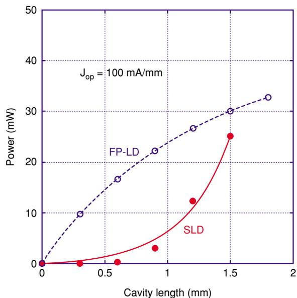
Fig. 3. Correlation between output power and cavity length.
