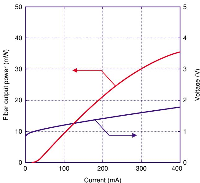
Fig. 7. Typical light-output power and voltage/current characteristics of SLD module.
