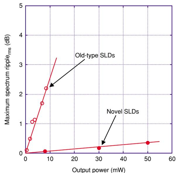
Fig. 2. Correlation between maximum spectrum ripple and chip output power.
