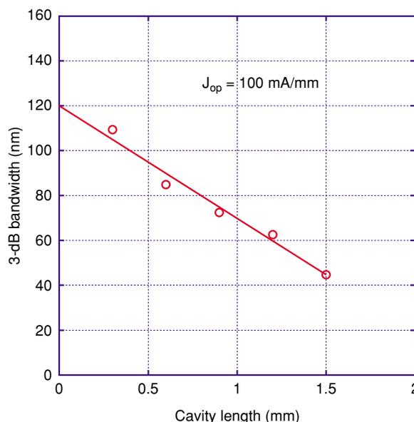
Fig. 4. Correlation between 3-dB bandwidth and cavity length.
