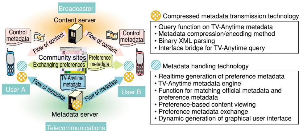
Fig. 3. Use scenario of metadata compression/handling technology.
