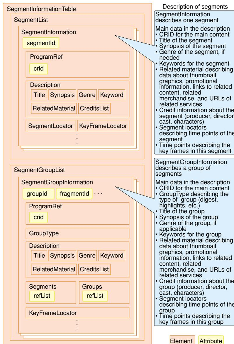
Fig.1. Structure of TV Anytime segment metadata.
