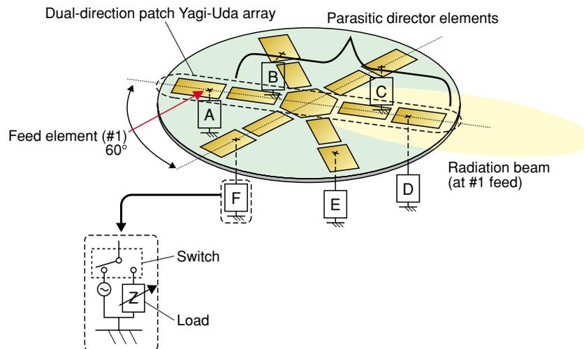
Fig. 9. Thin and small sector beam antenna.
