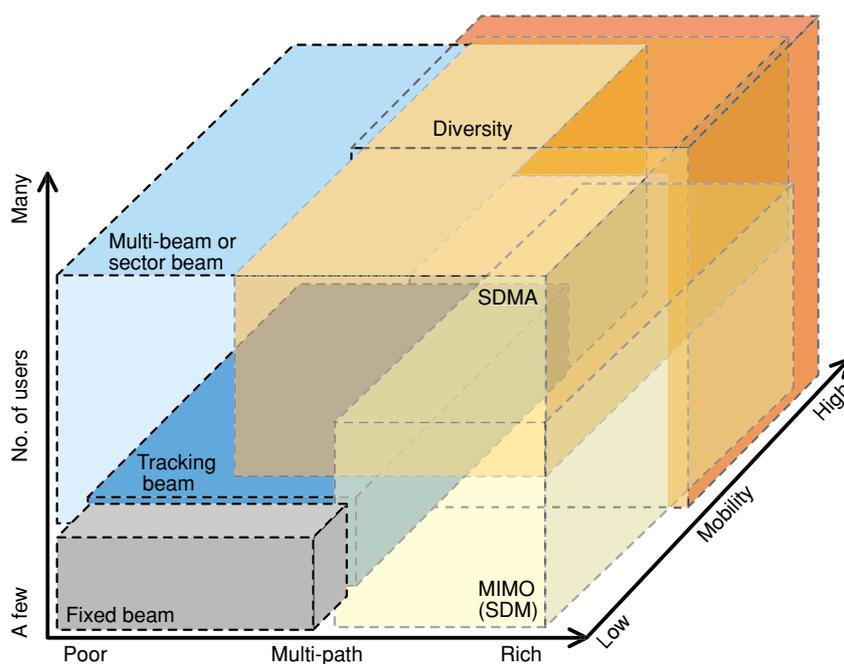
Fig. 8. Dependence of multi-antenna techniques on system characteristics.
