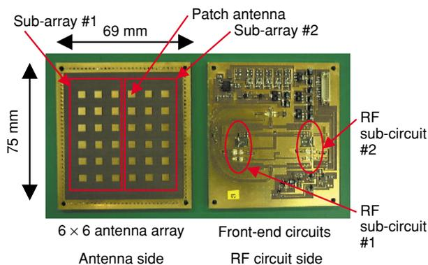
Fig. 7. Active integrated antenna for 25-GHz system.
