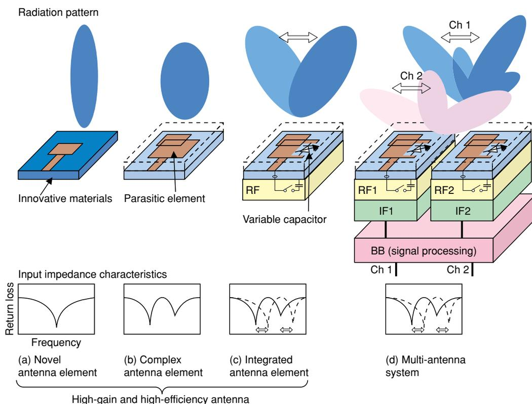
Fig. 4. Antenna elements and system.
