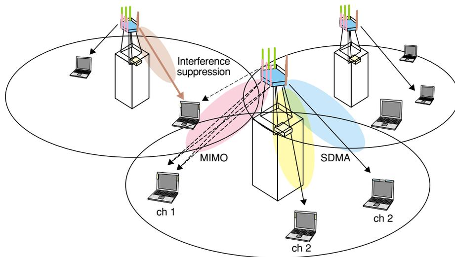
Fig. 5. Smart antenna system (land mobile telecommunication).
