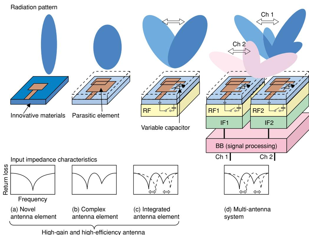
Fig. 4. Antenna elements and system.
