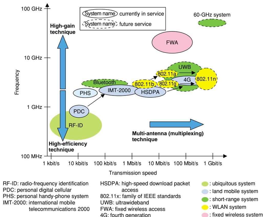
Fig. 2. Advances of terrestrial wireless communication systems and their relationship to antenna technologies.
