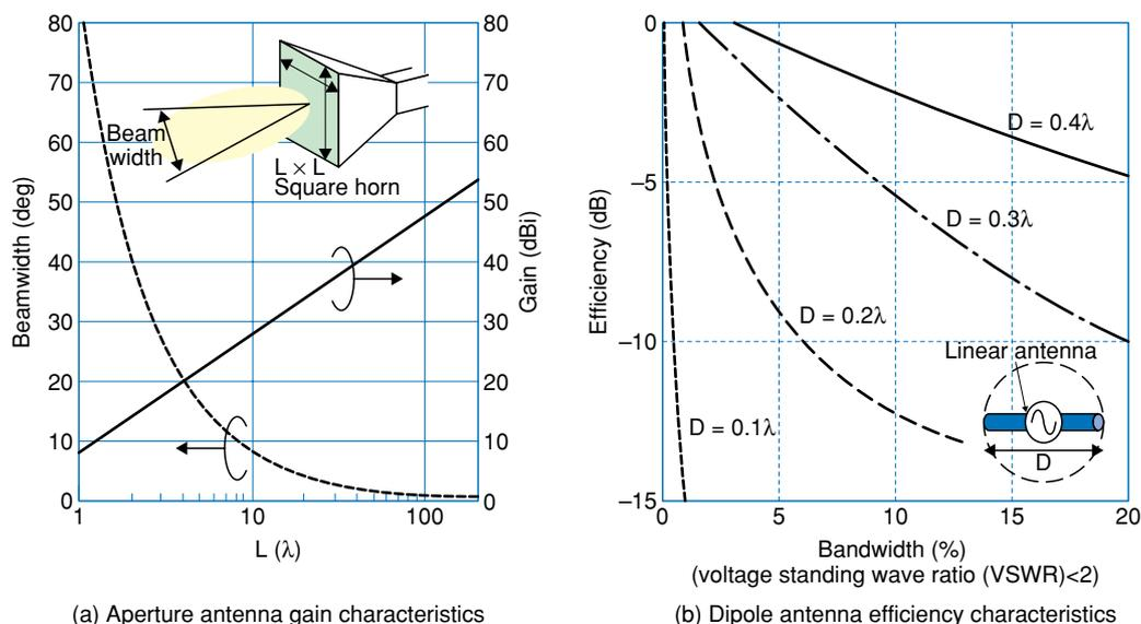
Fig. 3. Antenna gain and efficiency characteristics.
