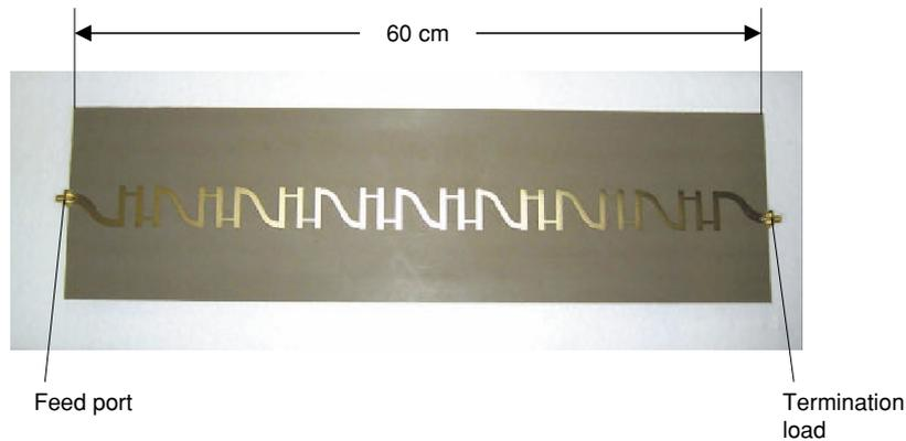
Fig. 12. Fabricated antenna.
