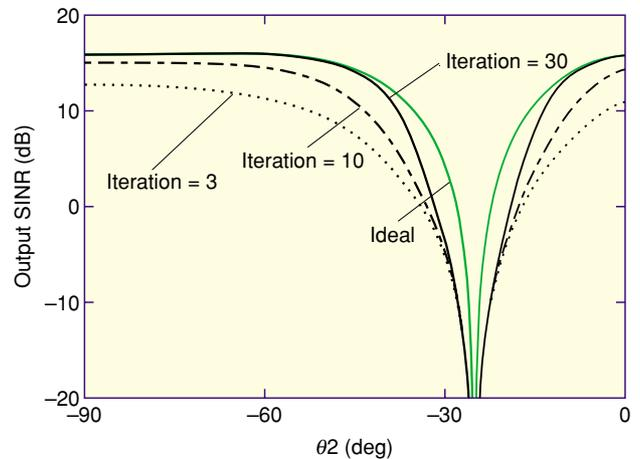
Fig. 12. SINR when a suboptimal approach is used.
