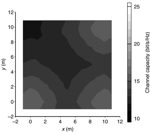
Fig. 6. Ergodic channel capacity distribution with a conventional scheme with four antenna branches at each AP.
