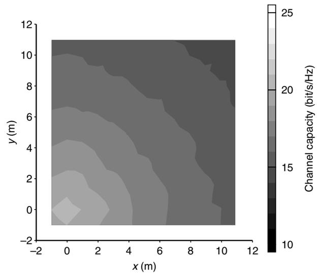
Fig. 7. Ergodic channel capacity distribution with a conventional scheme where 12 antenna branches are assumed at one AP.
