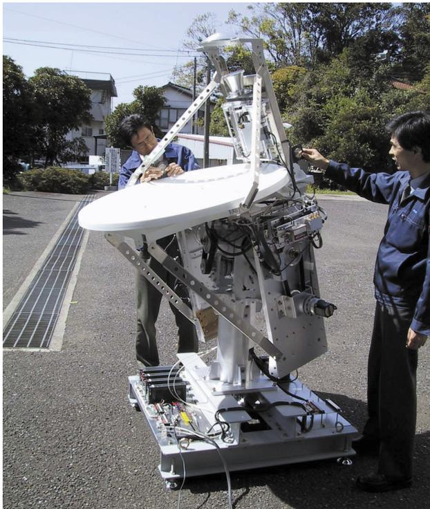
Fig. 10. Antenna system prototype.
